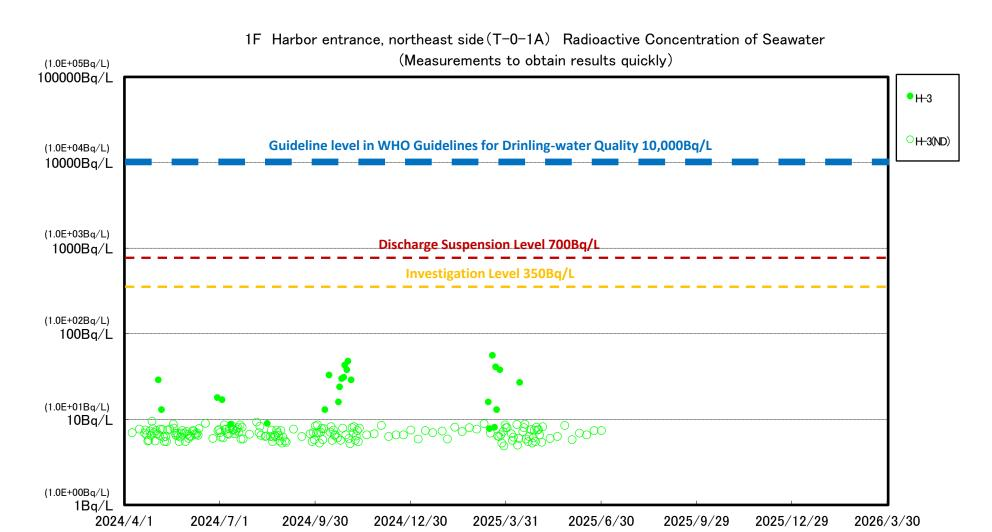
Discharge Suspension Level: Index for determining if discharge needs to be suspended. Investigation Level: Index for determining actions (inspection of facilities and operational procedures, increased monitoring, etc.) to be taken before the Discharge Suspension Level is reached.
