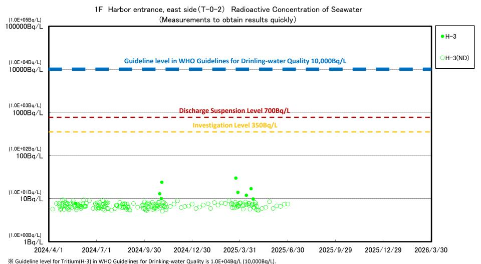
Discharge Suspension Level: Index for determining if discharge needs to be suspended.
