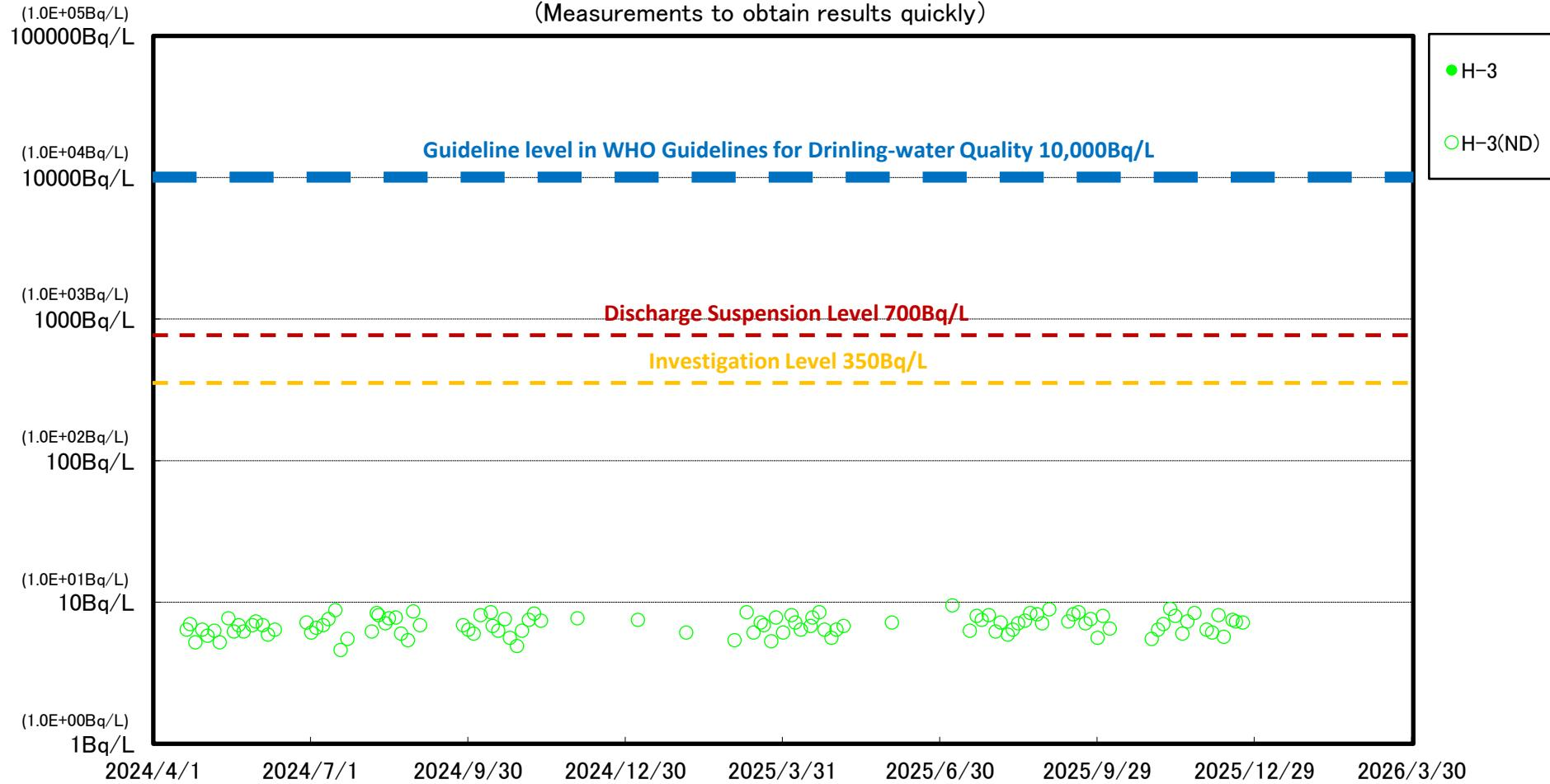
3km offshore of 1F site (T-D5) Surface layer Radioactive Concentration of Seawater
