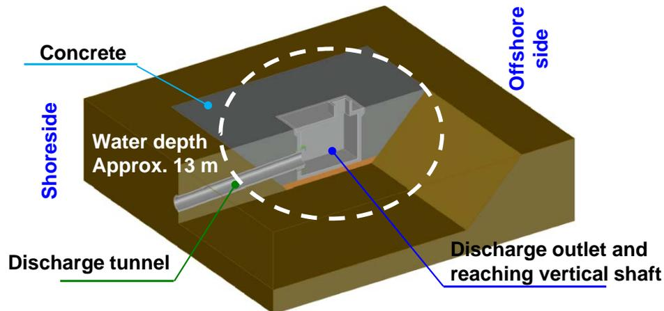
Image drawing of discharge outlet
