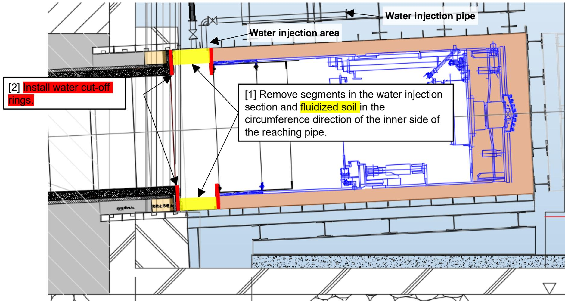
Image drawing of water cut-off (details)
