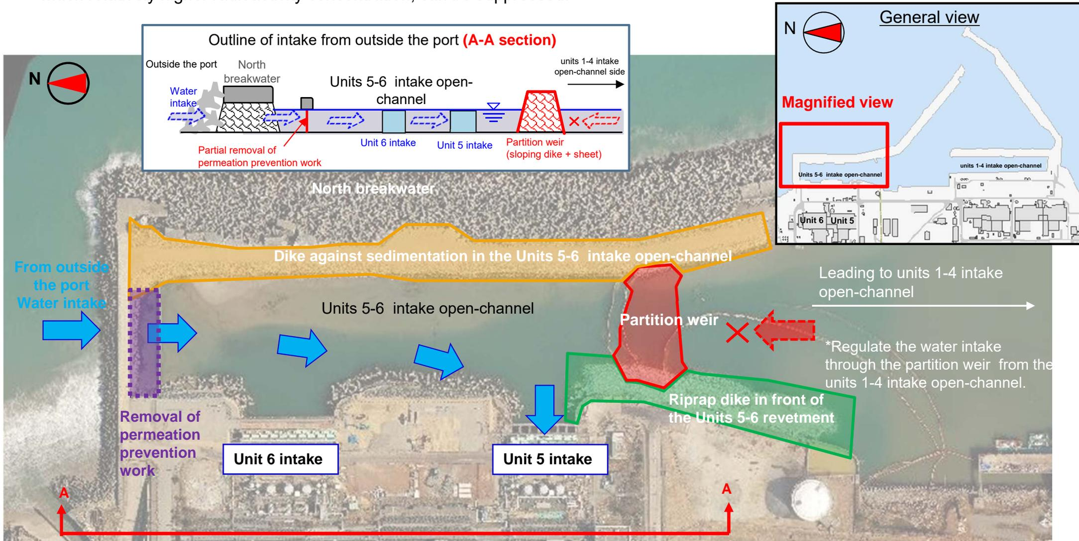
2-1(1) [3] Methods of seawater intake and discharging ALPS treated water after dilution
