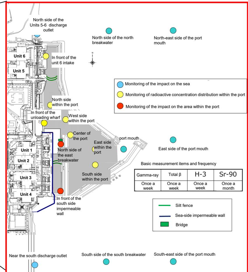
Figure: Location of marine monitoring around the plant
