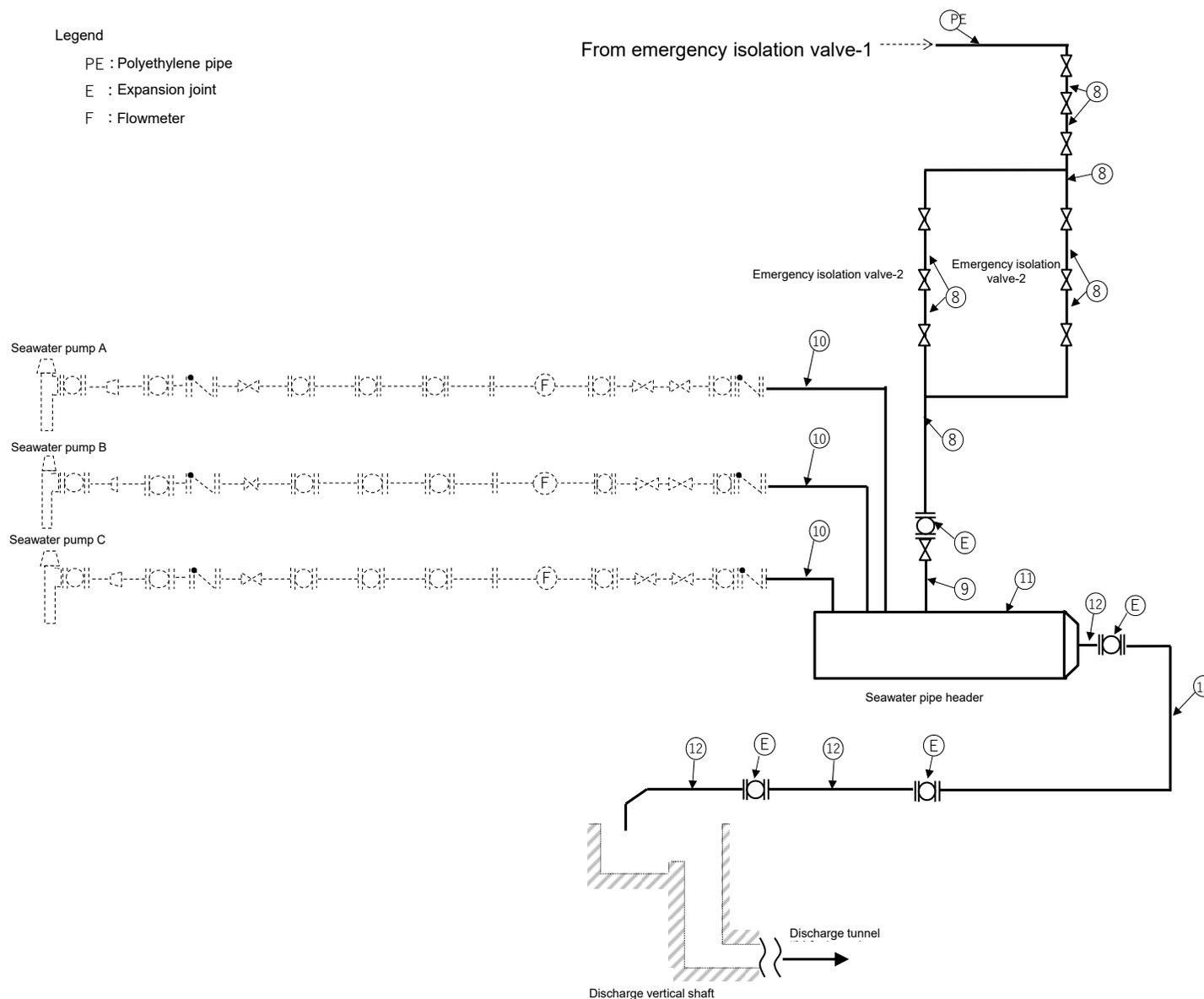
Figure-1 Piping diagram (5/5)
