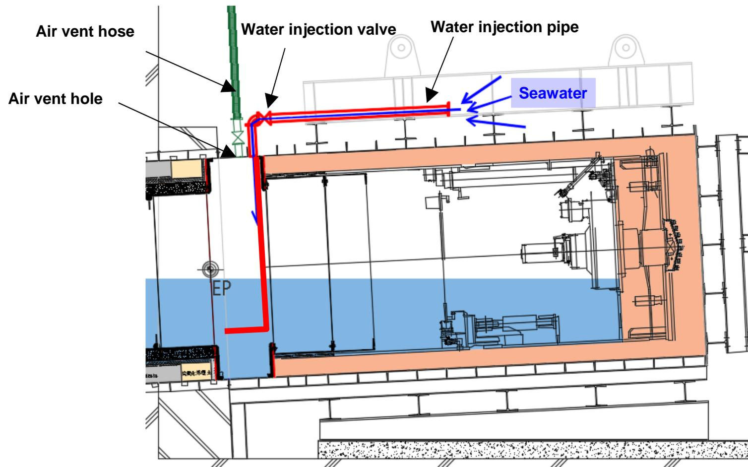
Image drawing of water injection work condition
