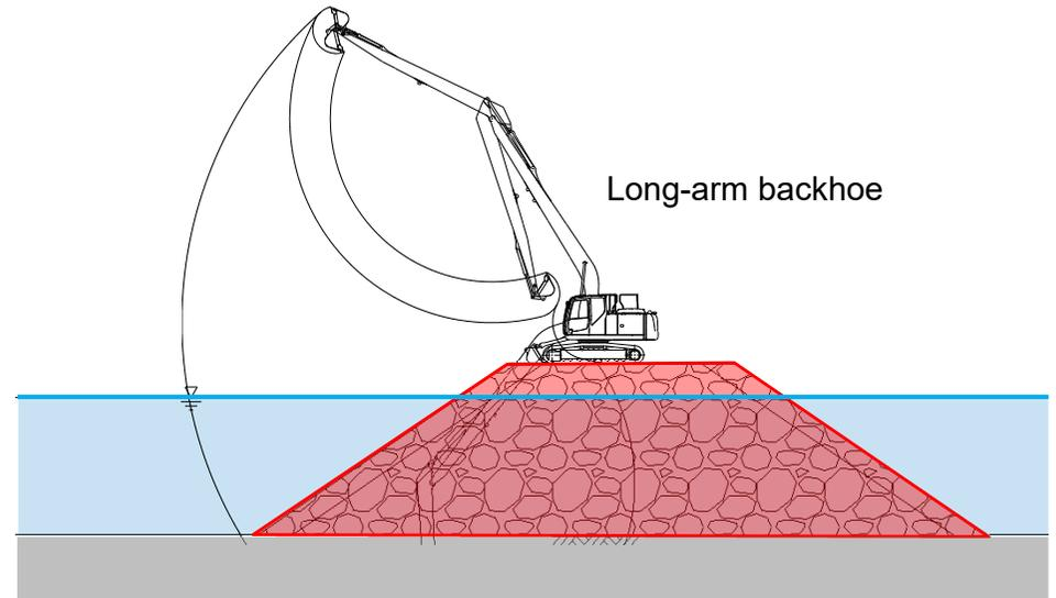
Image drawing of the construction of partition weir
