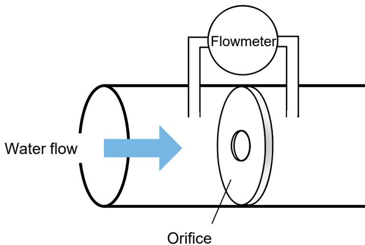
Image drawing of measurement with differential-pressure type flowmeter (orifice)
