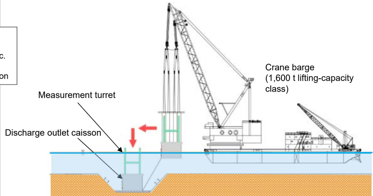
Image drawing of discharge outlet caisson installation (sectional view)
