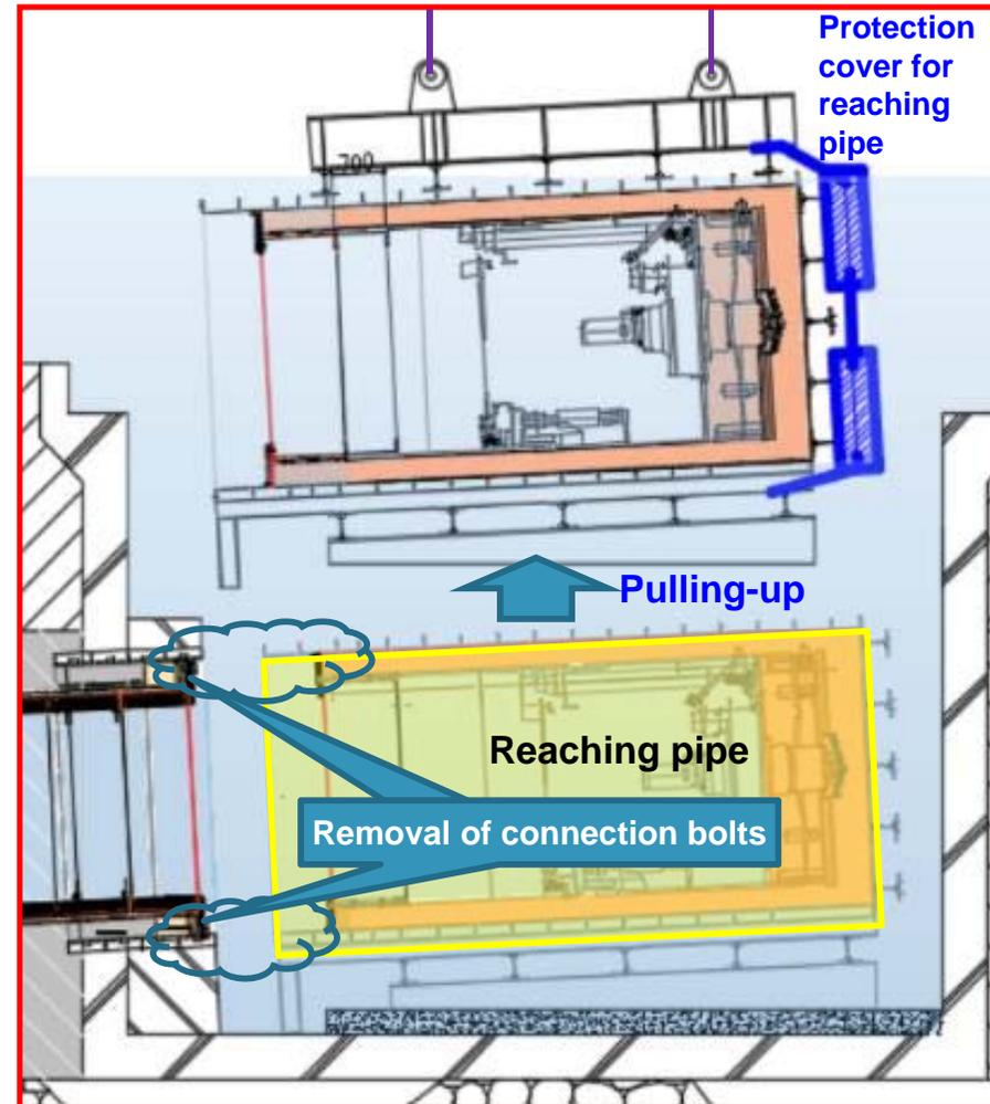
Image drawing of reaching pipe (shield machine) removal
