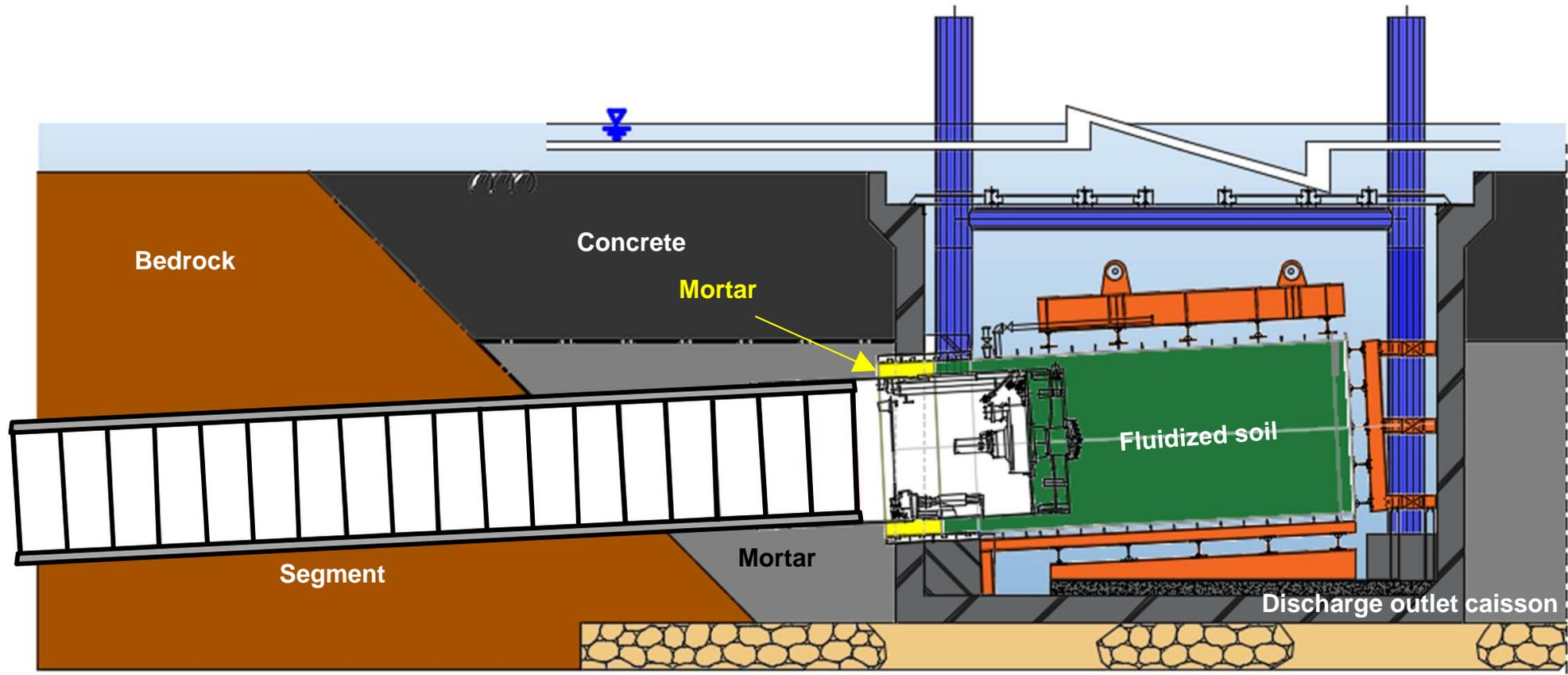
Image drawing of the shield machine reaching
