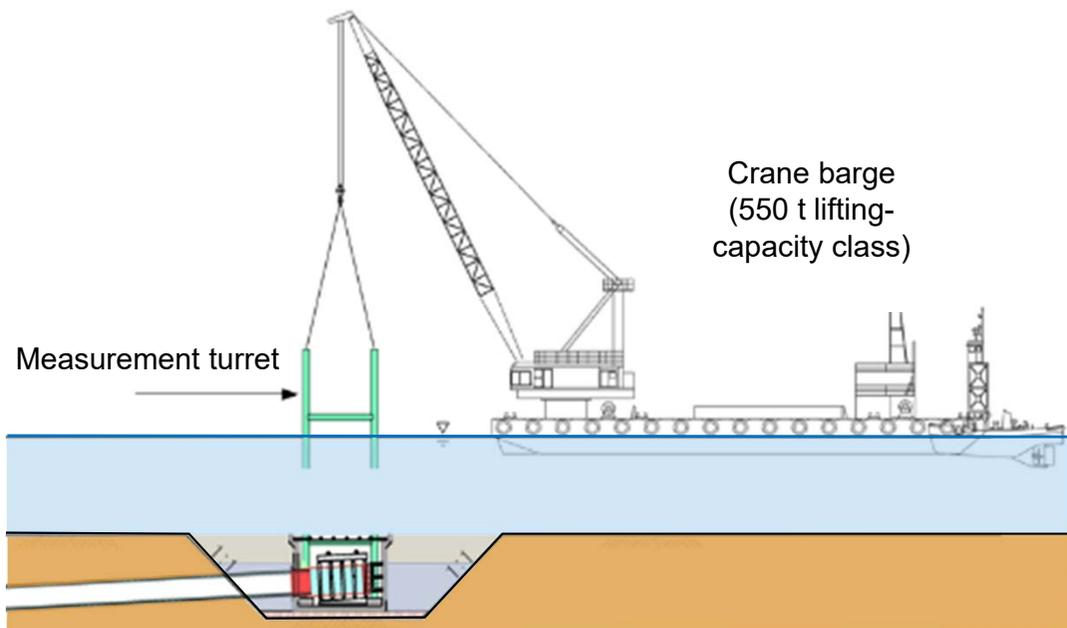
Image drawing of measurement turret removal
