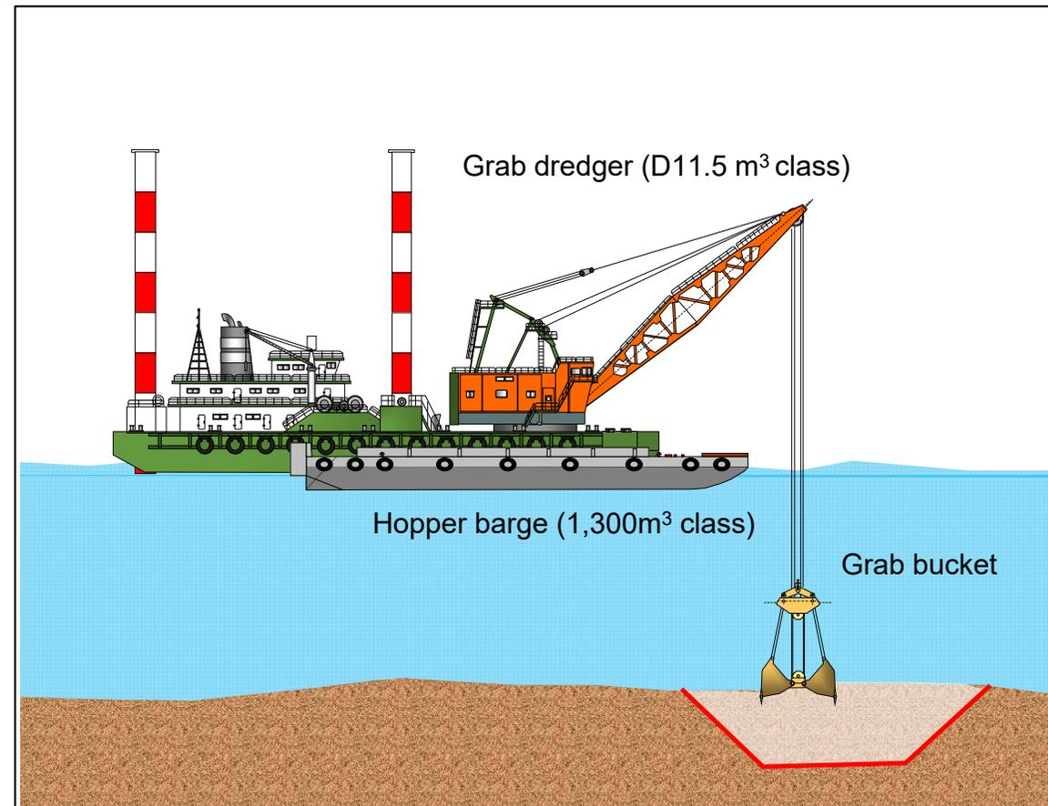
Image drawing of drilling at sea with grab dredger (sectional view)
