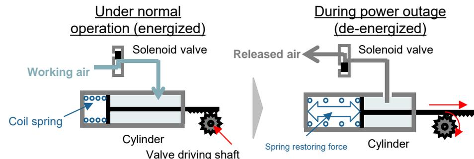
The cylinder is filled with air to maintain the valve "Open."
