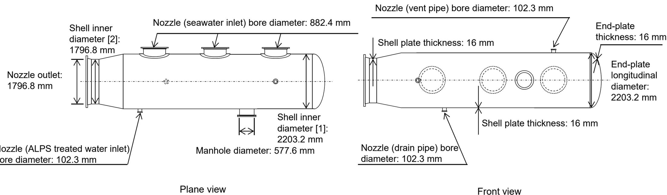
Structural drawing of seawater pipe header
