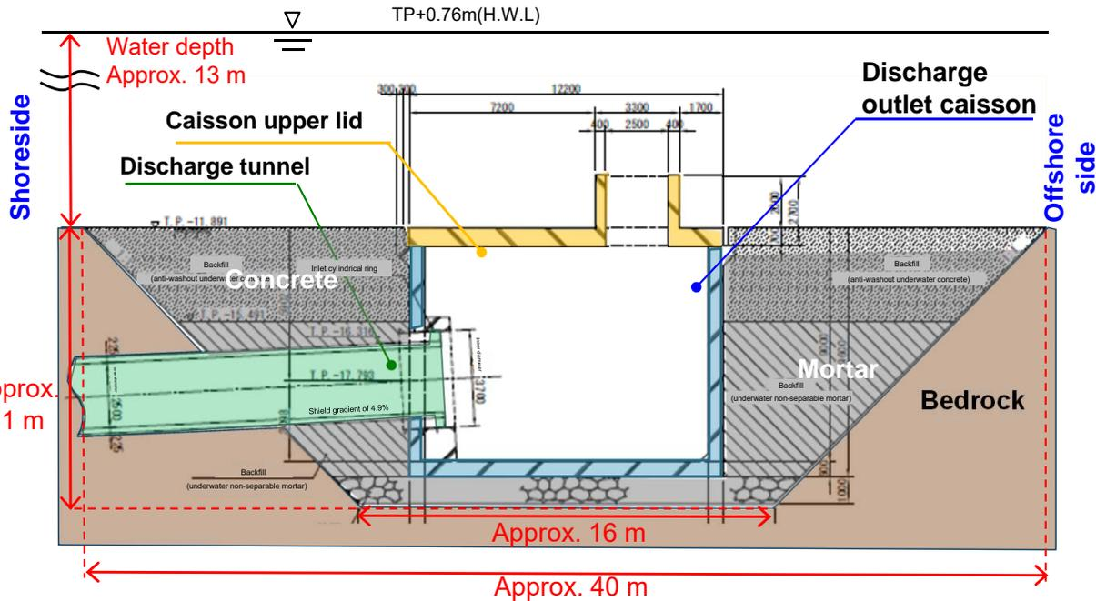
Image drawing of the discharge outlet cross-section
