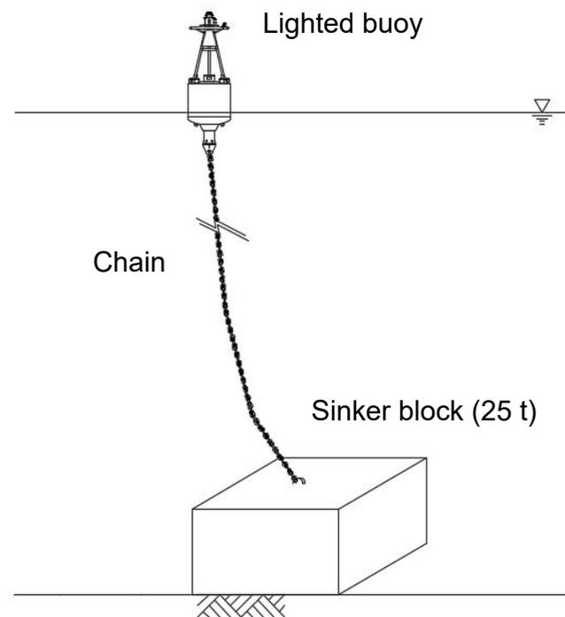
Image drawing of setting a lighted buoy
