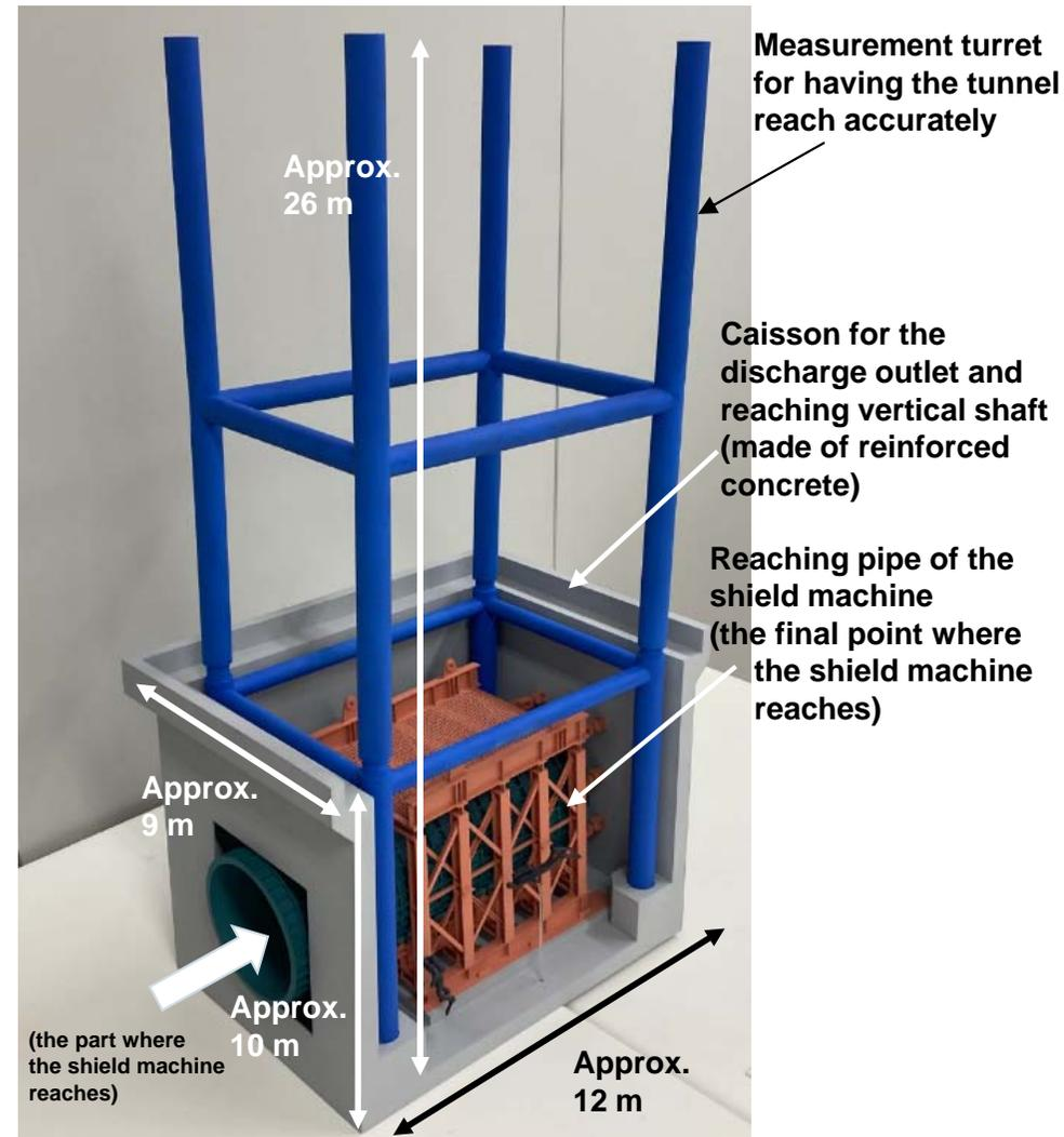
Image drawing of manufacturing discharge outlet caisson
