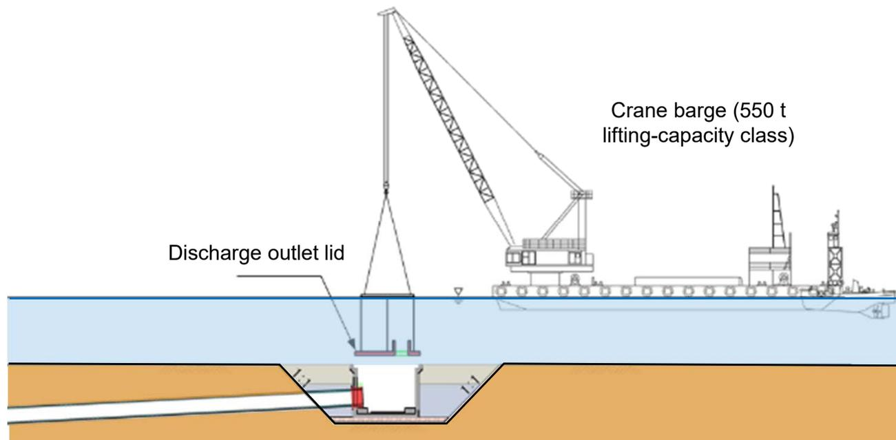
Image drawing of discharge outlet caisson lid installation
