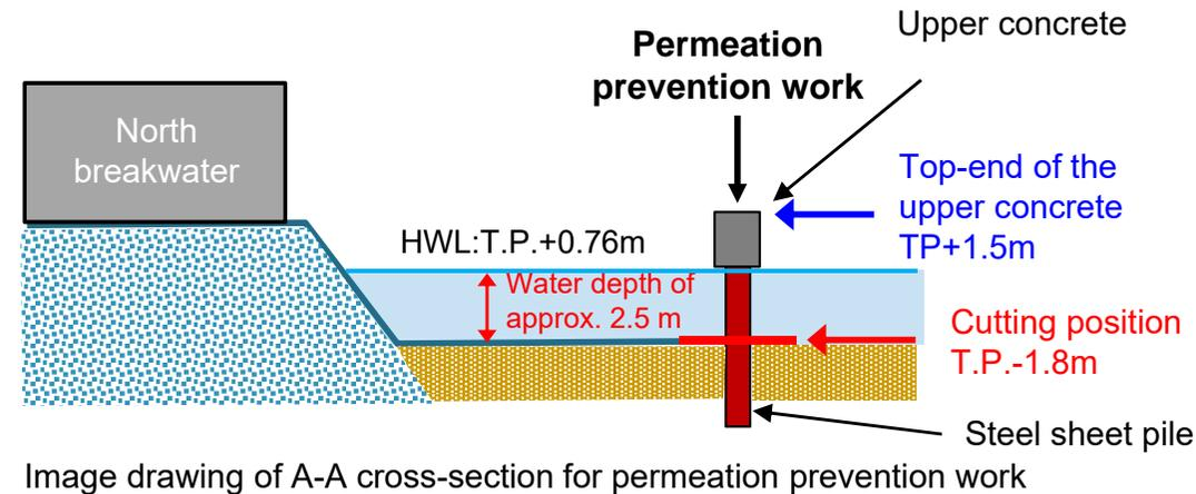
Image drawing of A-A cross-section for permeation prevention work
