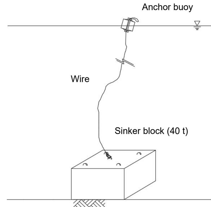
Image drawing of installing sinker blocks for mooring ships
