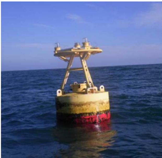
Image photo of a lighted buoy
