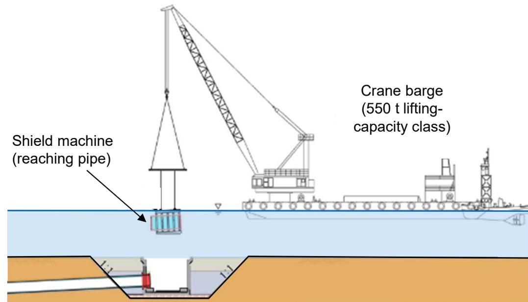
Image drawing of shield machine (reaching pipe) removal
