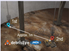
Fuel debris sampling site on the surface inside the Unit 2 pedestal
