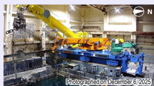
Entire fuel handling machine inside the Reactor Building
