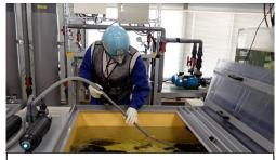
Underwater vacuum cleaner being used to remove residue and excrement
