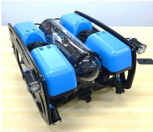
Commercially available submersible robot used as the platform
