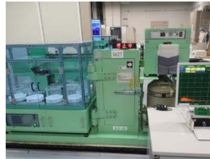
Reference: existing germanium semiconductor detector (Photo of the device in the chemical analysis building measurement room)
