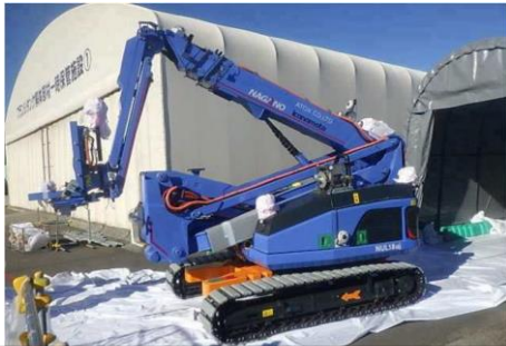
○ Elevated work platform truck Equipped a platform to carry the γ imager/ FirstLook/ SPOT to each floor
