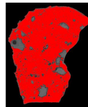
Image analysis example: Assessment of void area ratio
