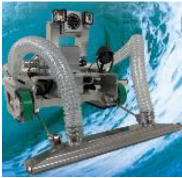
Submersible cleaning robot
