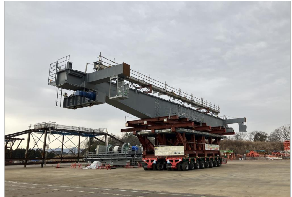
The rubble removal overhead crane loaded onto the super carrier
