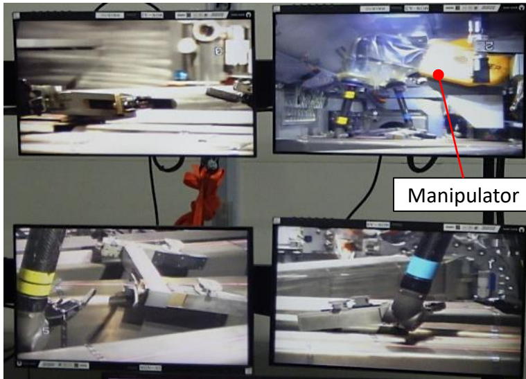
Performing an investigation with the manipulator (Monitors showing the camera feed from inside the enclosure)
