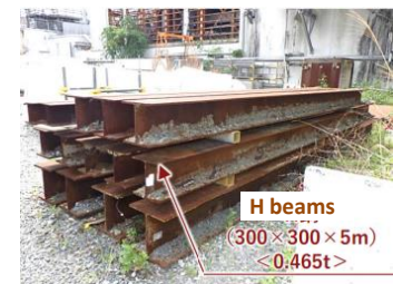
Remaining objects (H beams)
