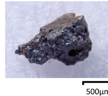
measurement location 1: Coarse U-Zr-O phase
