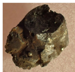
External view of the first fuel debris sample received by the NDC
