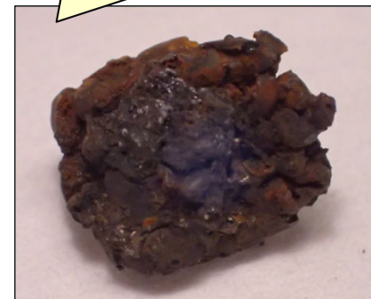
(Approx. 9mm×Approx. 7mm) 1st Fuel debris
