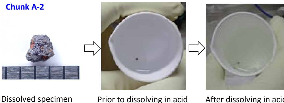
Figure Dissolving with nitric acid and a small amount of hydrofluoric acid
