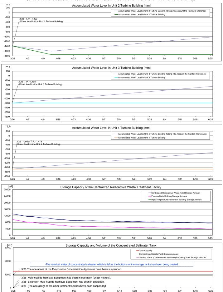
vore The amount of water treated through the 2nd Cesium Adsorption Apparatus is estimated to be 780m<sup>3</sup>/d (Subject to change depending on the factors such as the levels of water accumulated in T/Bs.) - "Accumulated Water Levels in Unit 2, 3 and 4 T/Bs" are simulated water levels in consideration of the change of the water levels caused by recent rainfall, inflow of groundwater, etc.
