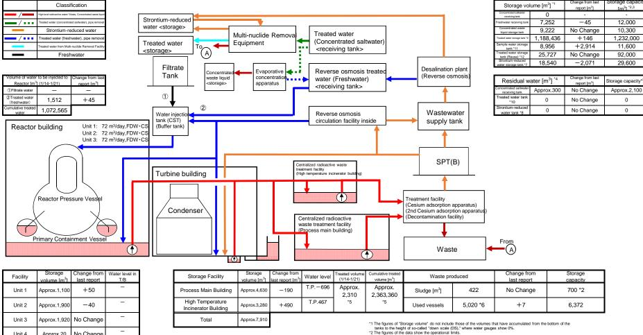
\*3 The figures of "Storage capacity" do not include those of the volumes that have accumulated from the bottom of the tanks to the height of so-called "down scale (DS)," where water gauges show 0%. However, each tank has the capacity that accommodates more than the storage volume that accumulates up to the height of "DS."
