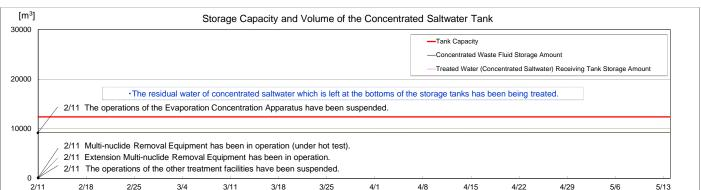
\*\*1 Storage place of water transported from the Units 1-4 will be changed over from the high temperature incinerator building to the process main building.
