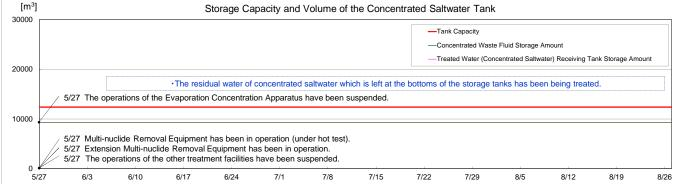
Note - The amount of water treated through the treatment facilities is changed depending on the factors such as stored amount in the accumulated water storing facilities.
