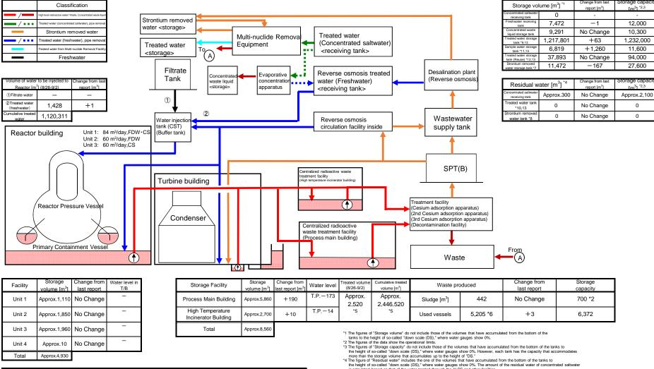
[Main operations that are planned to be conducted during the period from August 26, 2021 to September 2, 2021] Water transfer from the Units 1-4 to the buildings (Units 1-4, Centralized radioactive waste treatment facilities) and to the treatment facilities will
