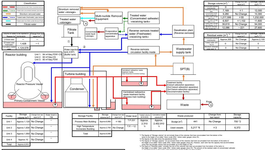
[Main operations that are planned to be conducted during the period from September 16, 2021 to September 23, 2021] Water transfer from the Units 1-4 to the buildings (Units 1-4. Centralized radioactive waste treatment facilities) and to the treatment facilities will
