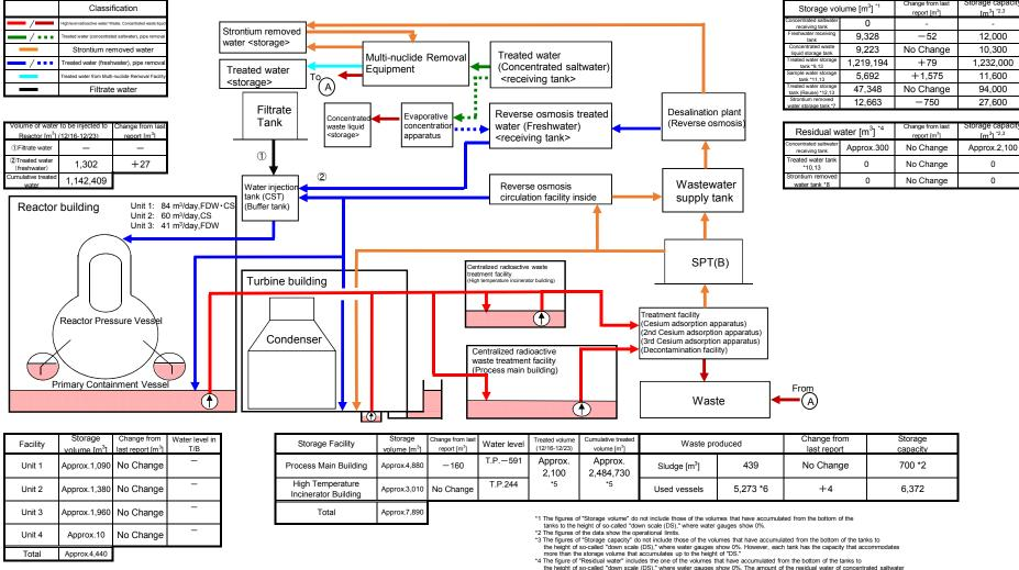
[Main operations that are planned to be conducted during the period from December 16, 2021 to December 23, 2021] Water transfer from the Units 1-4 to the buildings (Units 1-4. Centralized radioactive waste treatment facilities) and to the treatment facilities will be conducted whenever necessary
