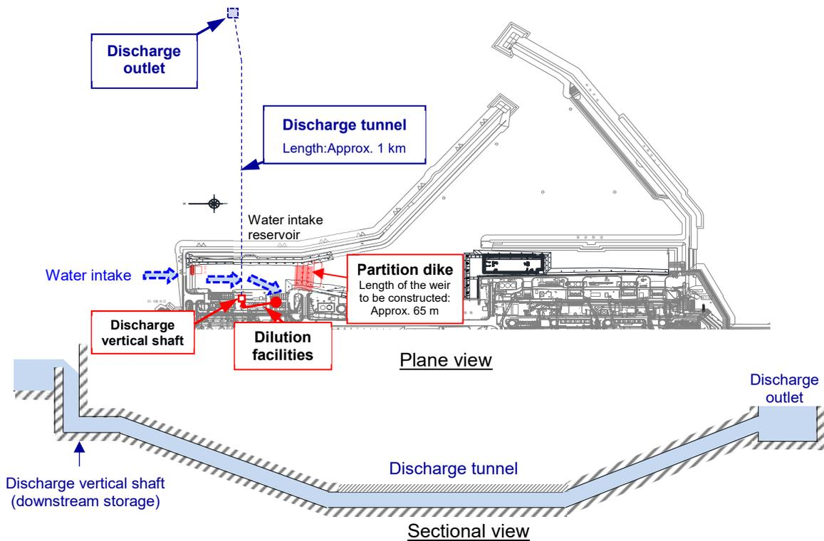
**Figure 4-2-2 Overall view of the intake and discharge facilities**
