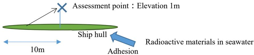
**Figure 4-4 Model for Assessment of Exposure from Ship Hull, Decommissioning Handbook**
