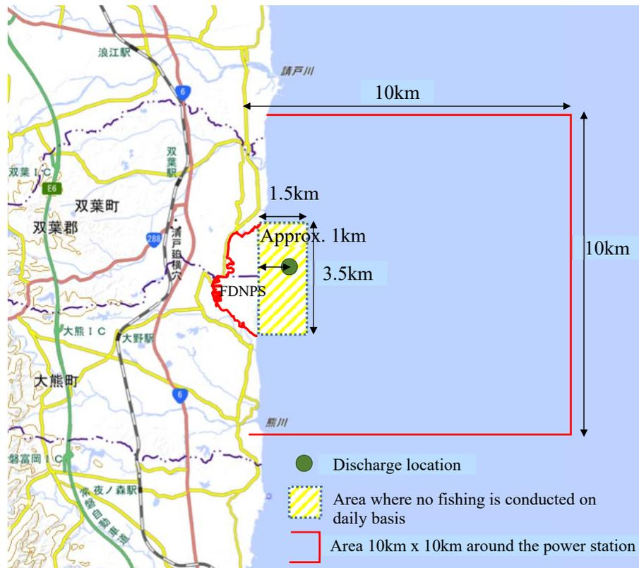
**Figure 4-3 Area Map for the Calculation of Concentration in Seawater for Assessment**
