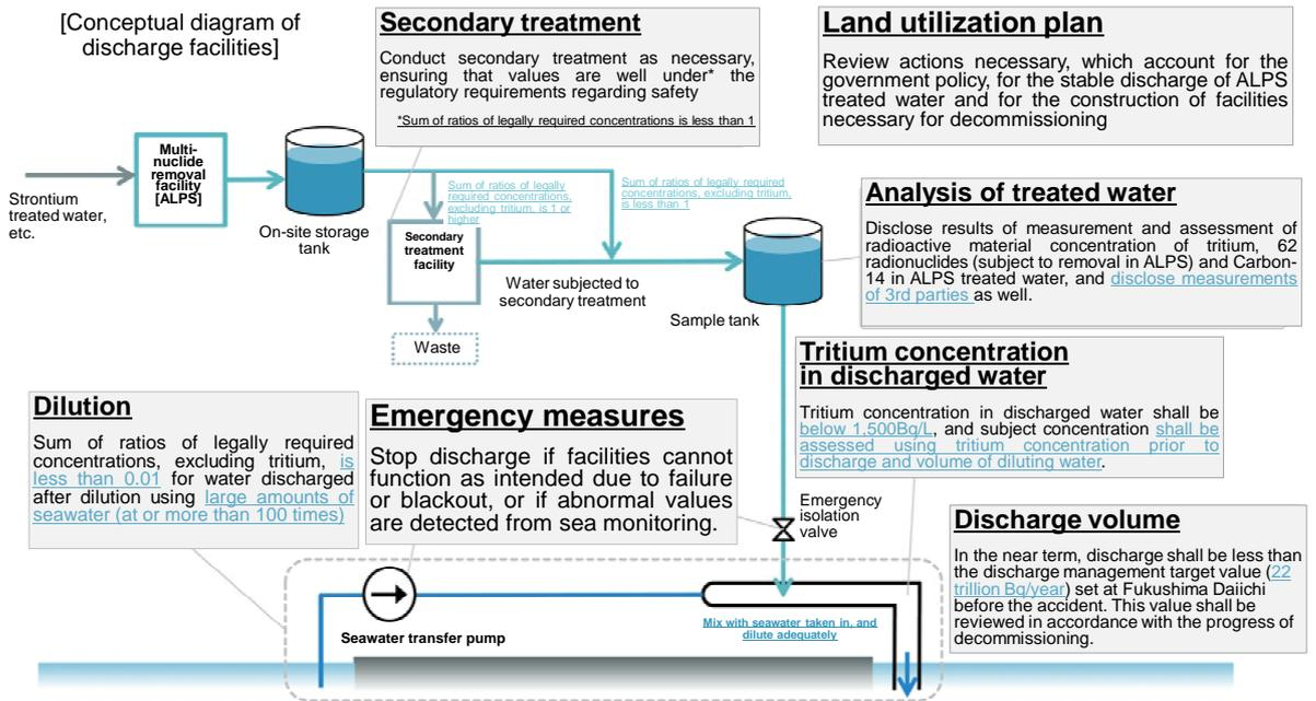
Figure 3-1 Schematic Drawing of Facilities for Discharge into the Sea
