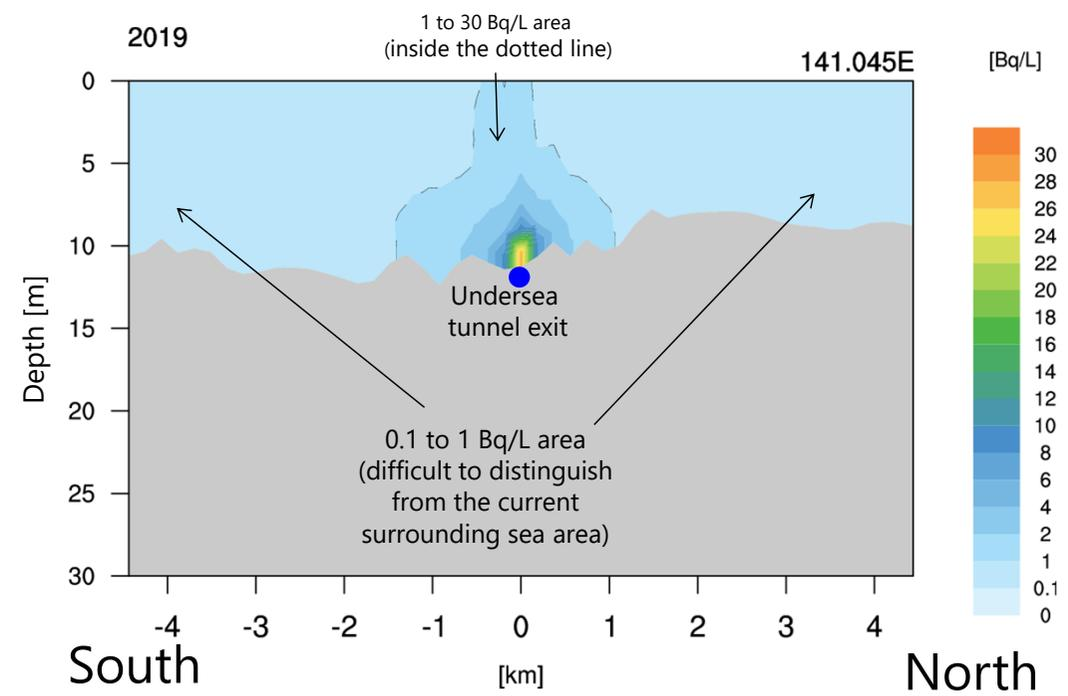
Cross-section view of the tunnel exit (North to south)
