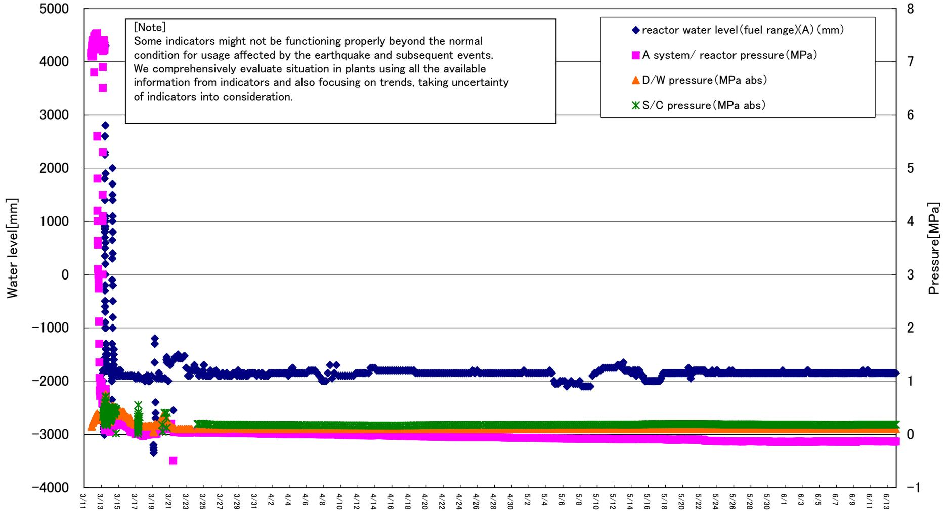
Fukushima Daiichi Nuclear Power Station Unit3 Parameters of Water level and Pressure
