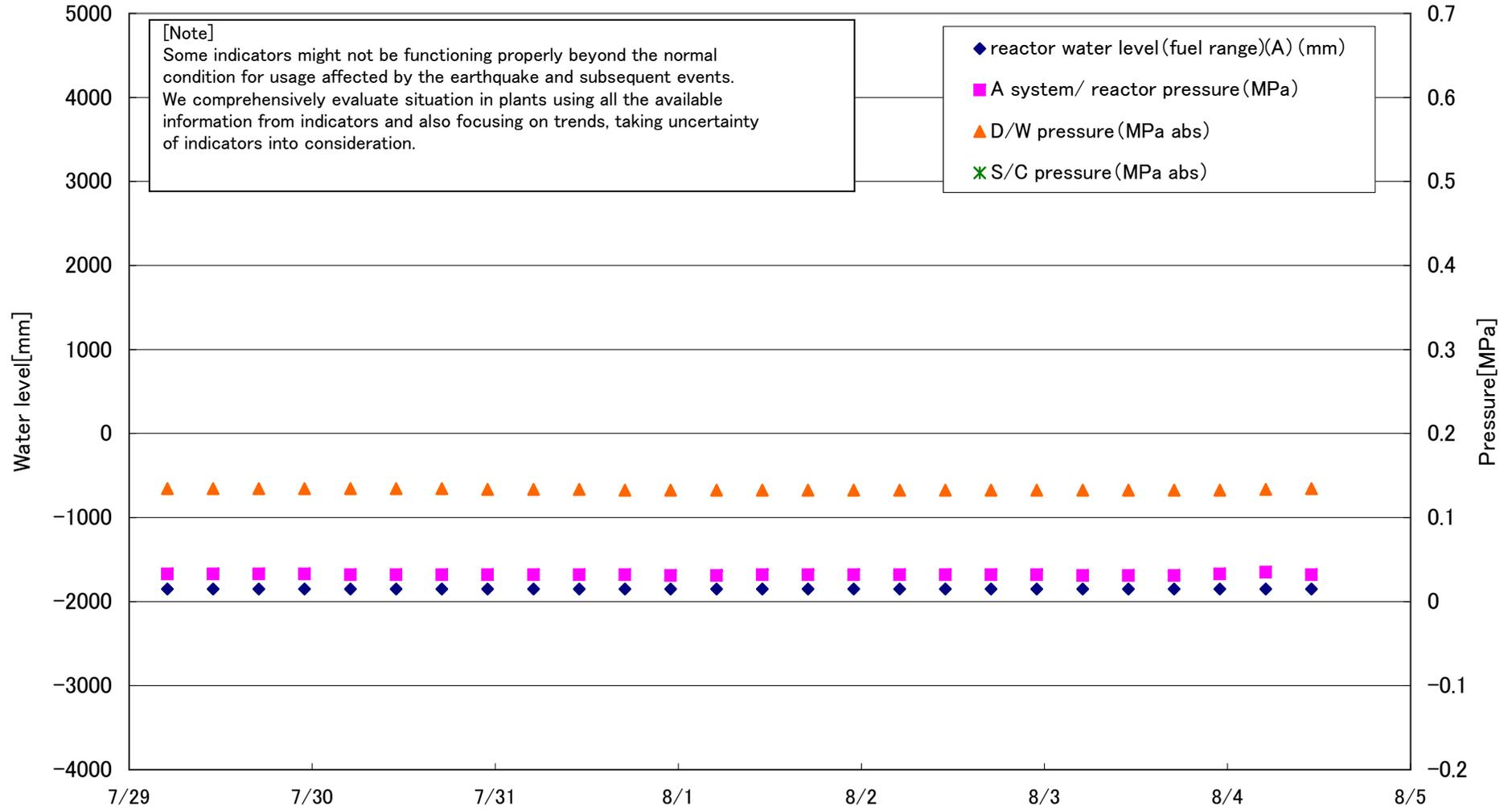
Fukushima Daiichi Nuclear Power Station Unit2 Parameters of Water level and Pressure
