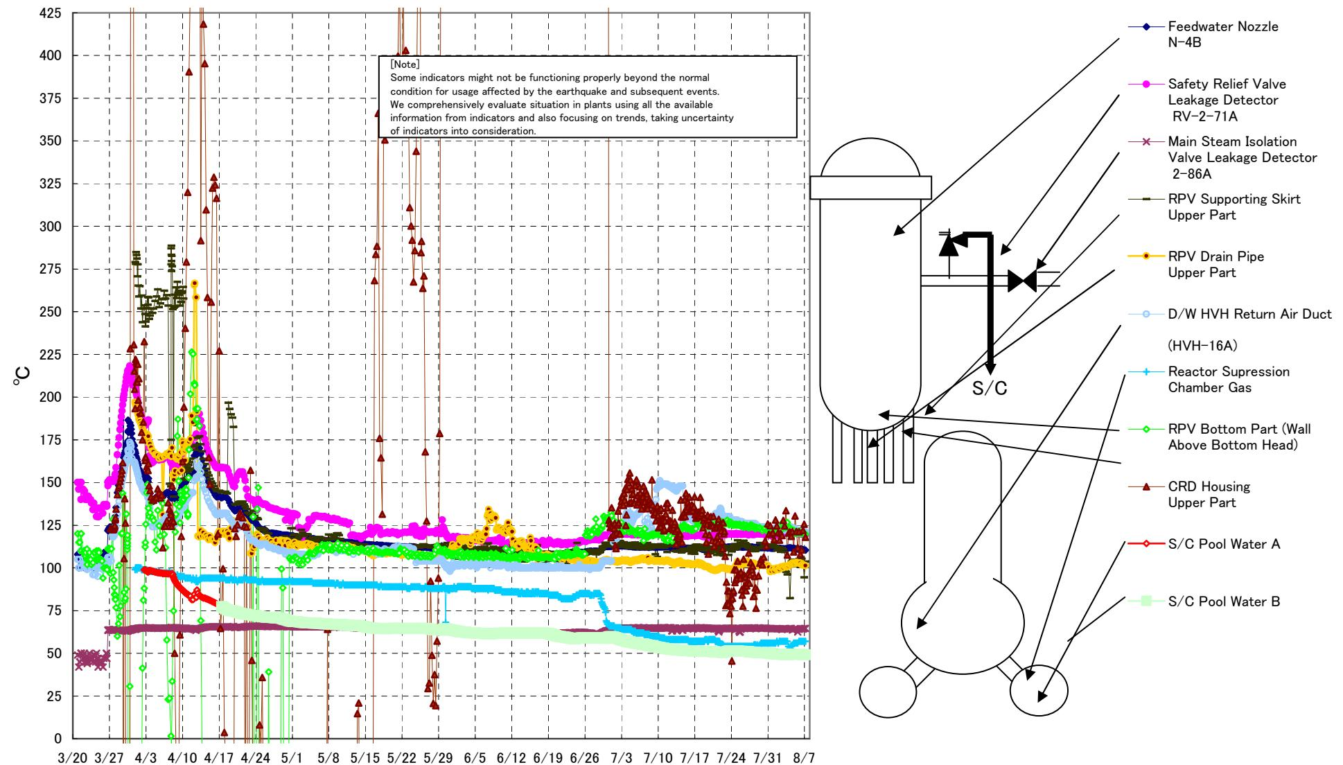
Fukushima Daiichi Nuclear Power Station Unit1 Parameters of Temperature
