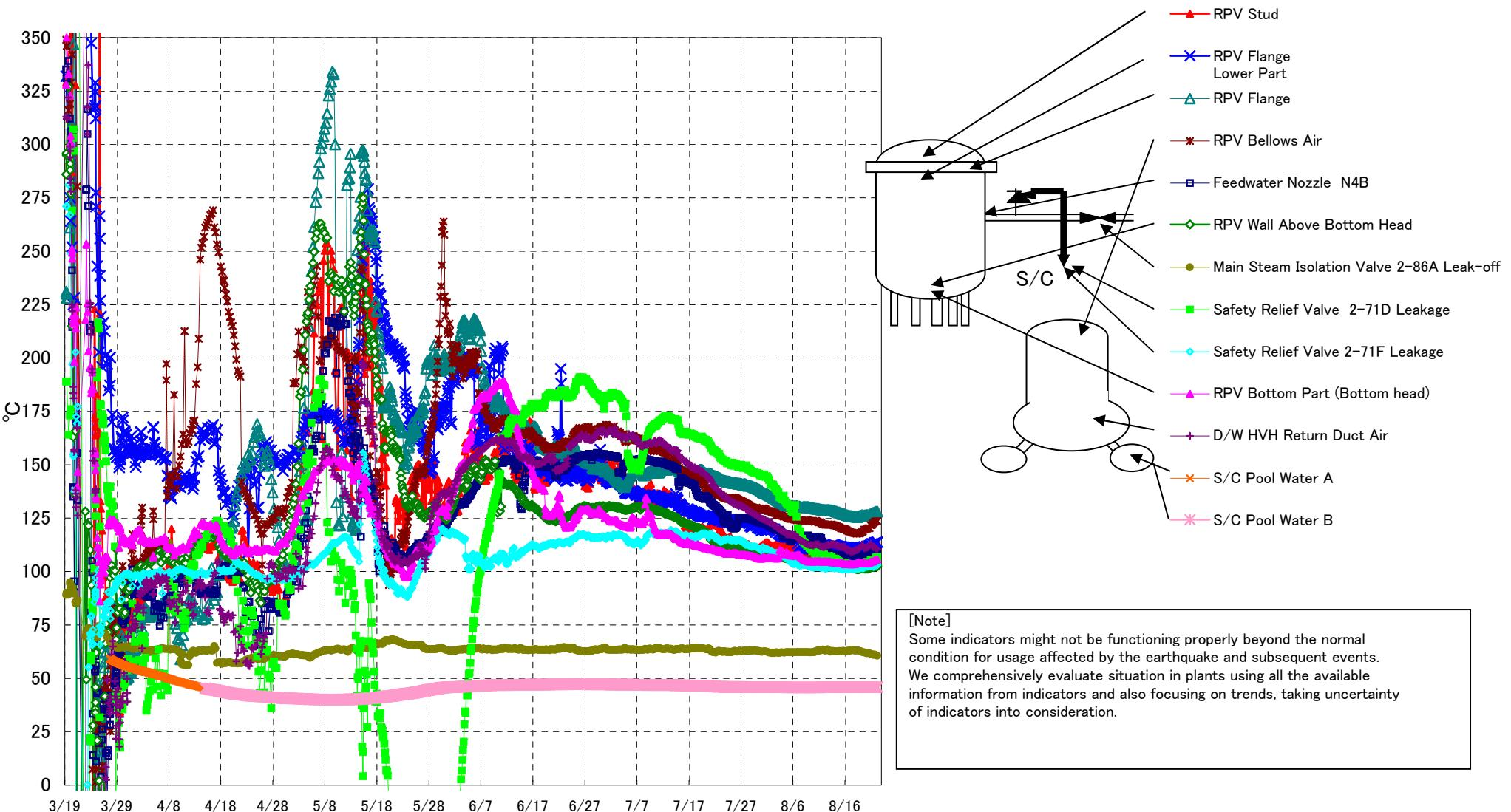
Fukushima Daiichi Nuclear Power Station Unit3 Parameters of Temperature
