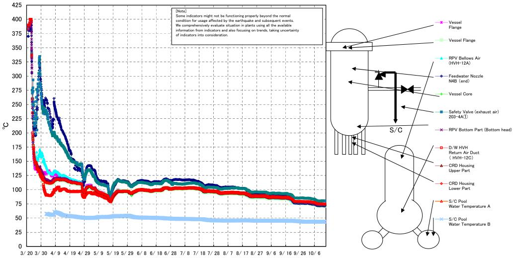
Fukushima Daiichi Nuclear Power Station Unit 1 Parameters of Temperature (Feedwater Nozzle and Safety Valve (Exhaust Air))
