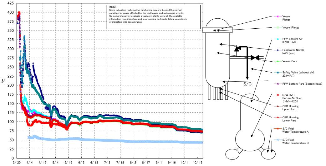
Fukushima Daiichi Nuclear Power Station Unit 1 Parameters of Temperature (Feedwater Nozzle and Safety Valve (Exhaust Air))
