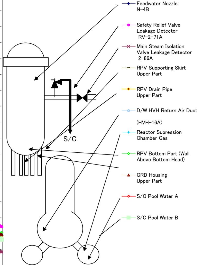
Fukushima Daiichi Nuclear Power Station Unit2 Parameters of Temperature
