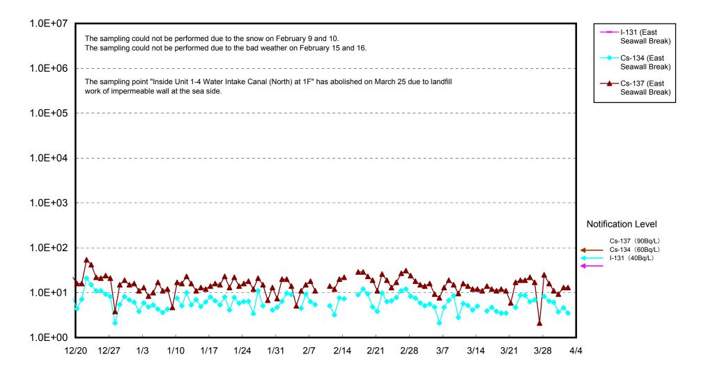
Radioactivity Density of the Seawater Obtained at Unit 2 Screen in Fukushima Daiichi NPS (Bq/L)
