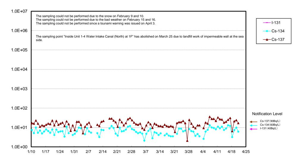
Radioactivity Density of the Seawater Obtained at Unit 3 Screen in Fukushima Daiichi NPS (Bq/L)
