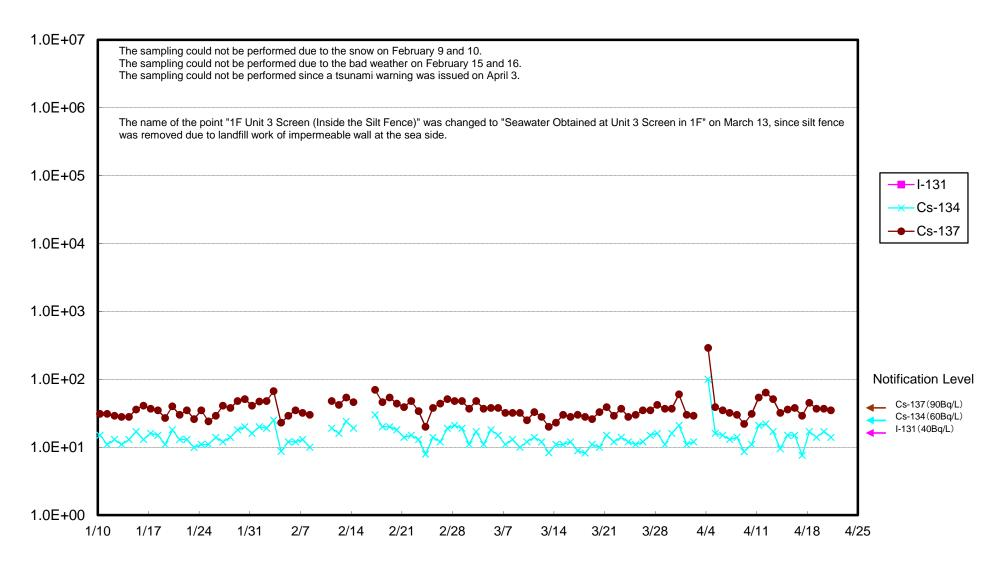
Radioactivity Density of the Seawater at Unit 4 Screen at 1F (Outside the Silt Fence) (Bq/L)
