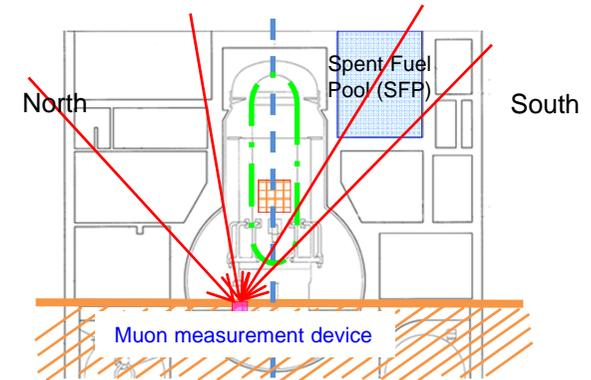
Measurement image of muon particles that pass through the reactor building (North-south cross section)
