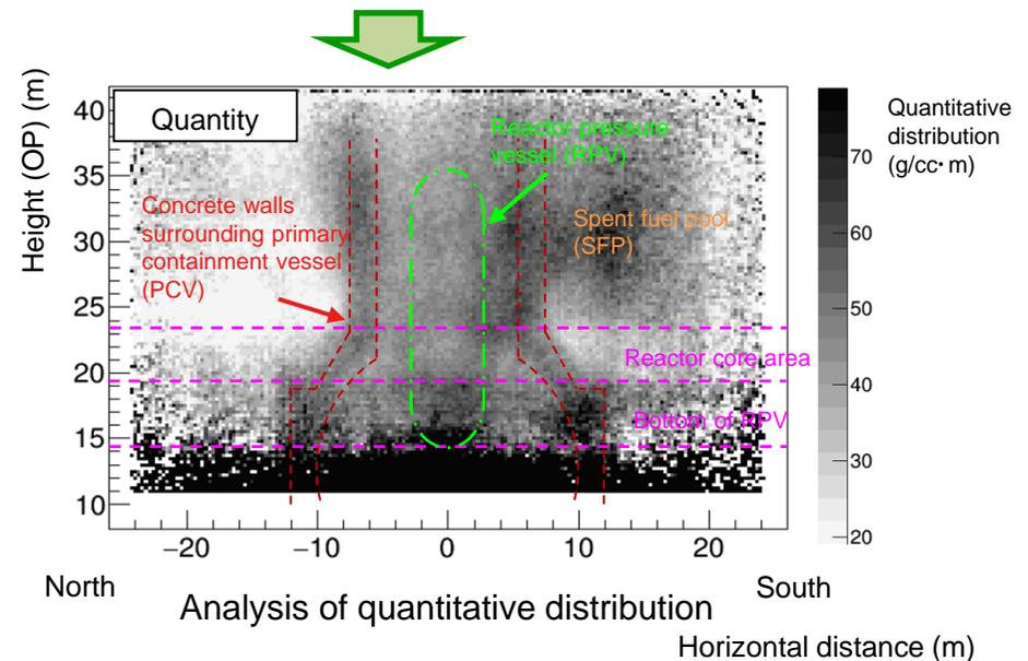
\*Shadows of concrete walls surrounding around the primary containment vessel were captured at the same height as the bottom of the reactor pressure vessel (around OP14.3m), which can be considered as significant shadows.
