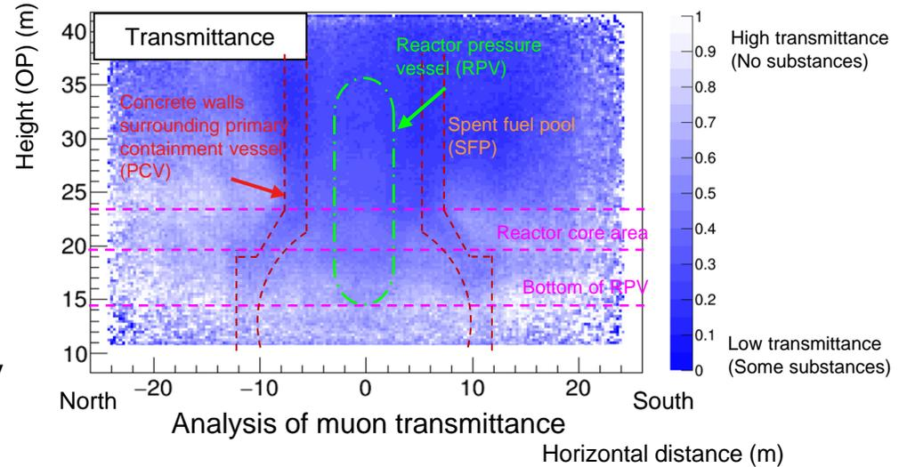
Quantitative distribution was analyzed from muon transmittance, considering the dependence on angles of muon transmittance based on the vertical difference in energy distribution of muon (the tendency that the color looks darker toward the upper part).
