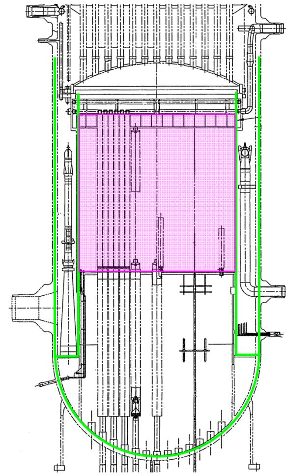
Structures at the lower part of the reactor pressure vessel
