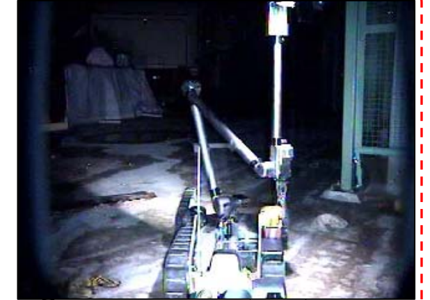
①Entrance of Airlock (North), R/B dose 84.9mSv/h , temp 29.2°C humidity 46.23% , O2 20.9%
