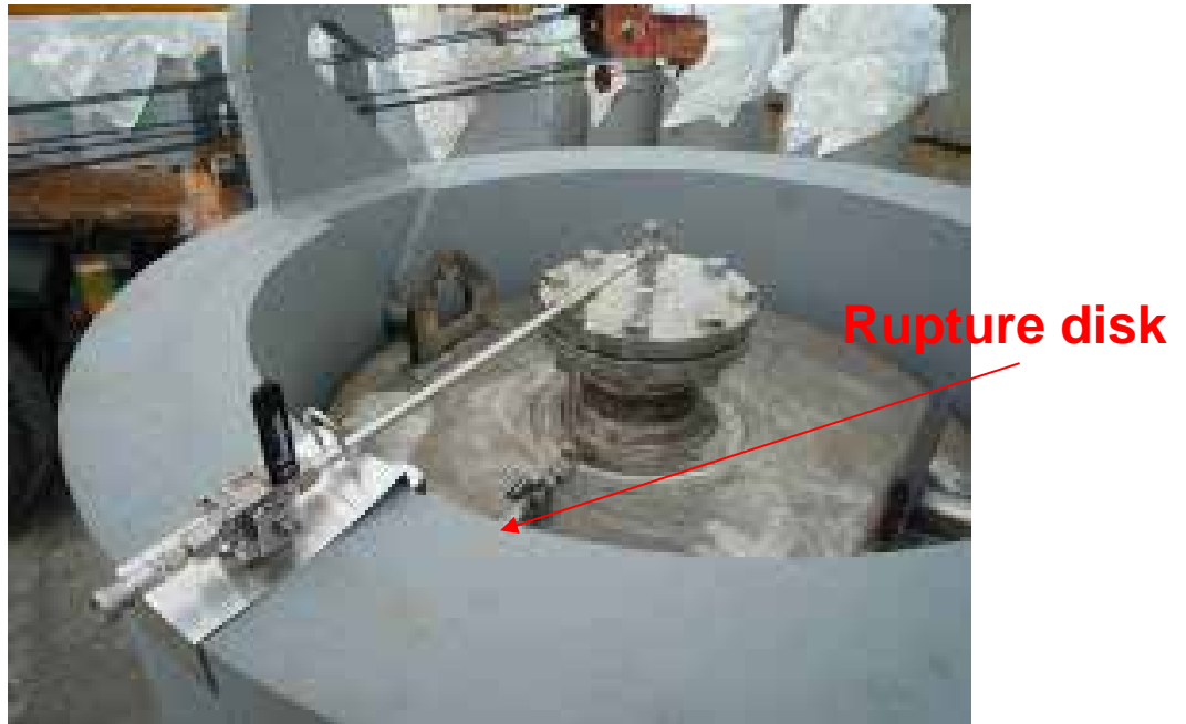
Rupture disk of cesium adsorption Instruments' vessel manufactured by Kurion
