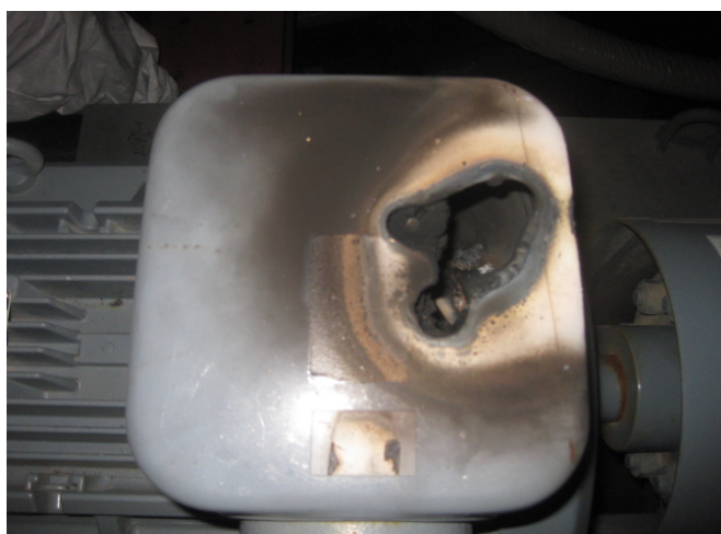
Upper part of the motor terminal
