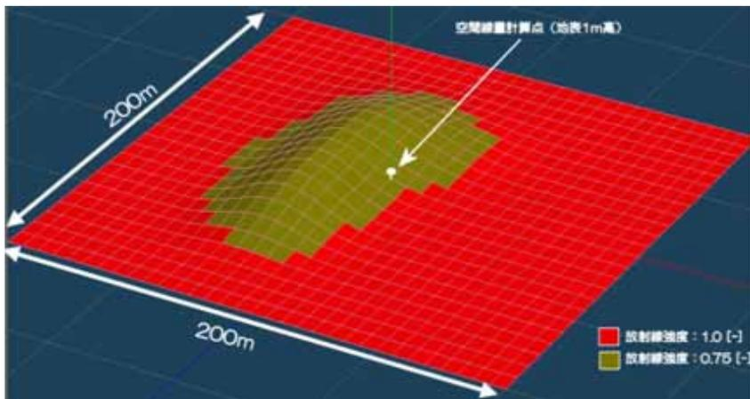
Settings of shape and radiation source (After decontamination)
