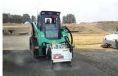
5. Asphalt surface cutting machine
