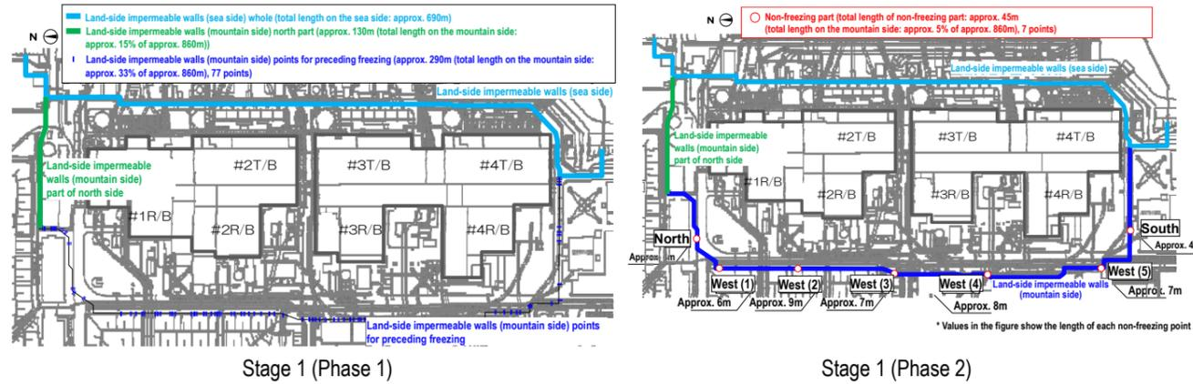
Figure 2: Scope of freezing of land-side impermeable walls
