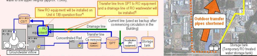
\*1 Unit 4 T/B operation floor is one of the installation proposals, which will be determined after further examination based on the work environment.
