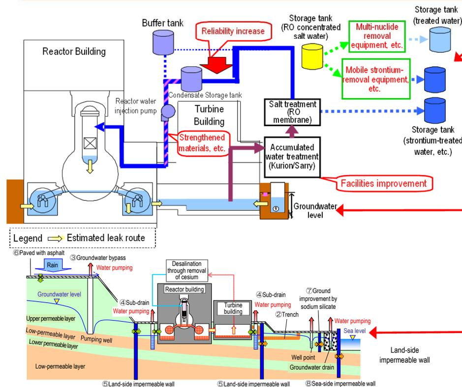
Preventing groundwater from flowing into the Reactor Buildings
