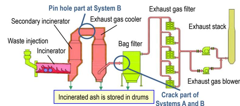
Figure 4: Overview of Radioactive Waste Incinerator
