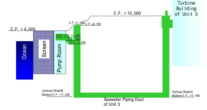
Seawater Piping Duct of Unit 3 Vertical Layout (b-b cross section view)
