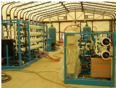
Water desalinations (RO membrane module)
