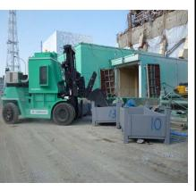
Packing into container bv a shielded forklift
