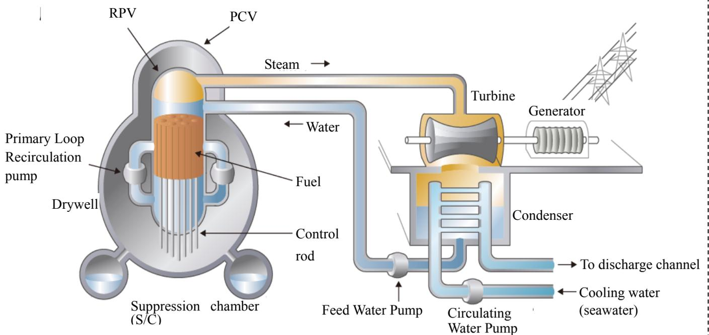
PCV: equipment that is consisted of the drywell (D/W) and suppression chamber (S/C)
