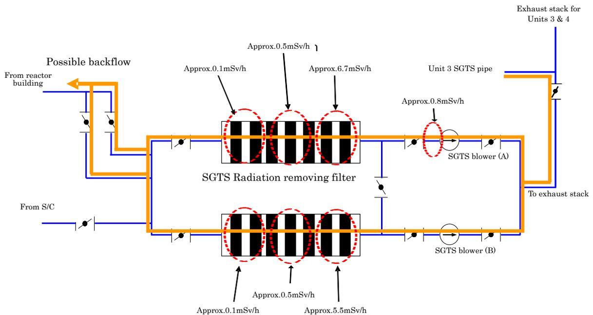
Results of measurement of amount of radiation in Unit 4 SGTS
