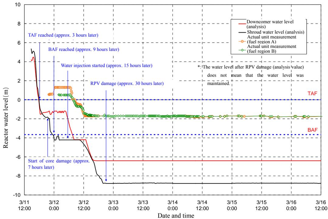
Changes in Unit 1 reactor water level (assuming that the IC was functioning temporarily)
