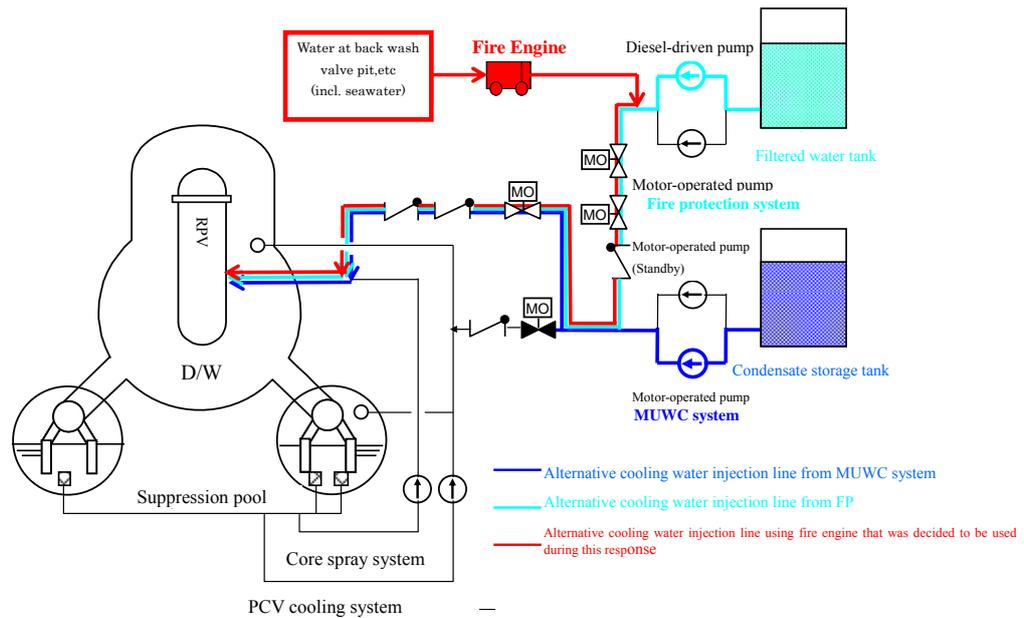
Alternative cooling water injection line
