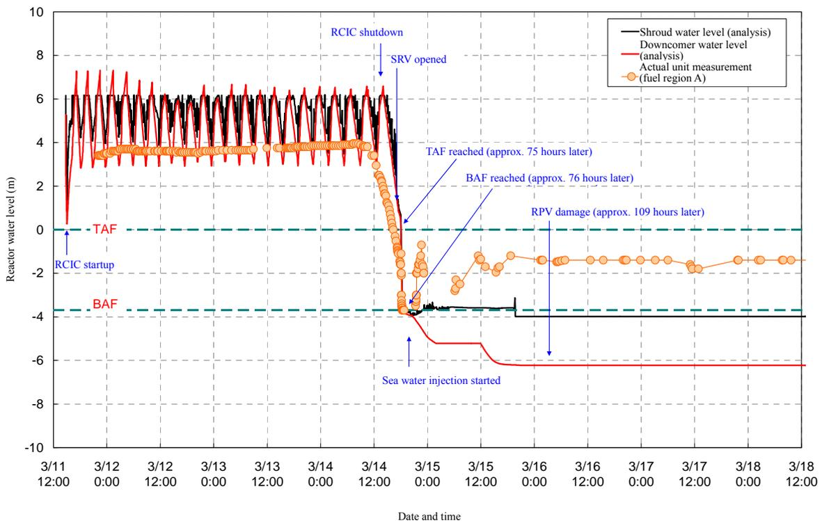
Unit 2 Change in reactor water level [Case 2]
