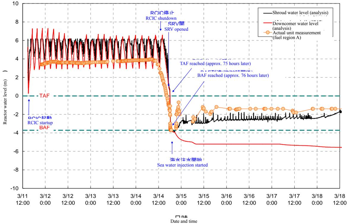
Unit 2 Changes in reactor water level [Case 1]
