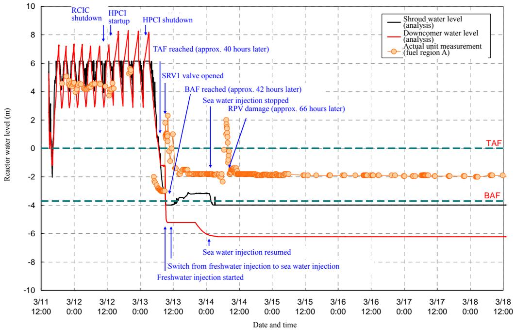
Unit 3 Changes in reactor water level [Case 2]
