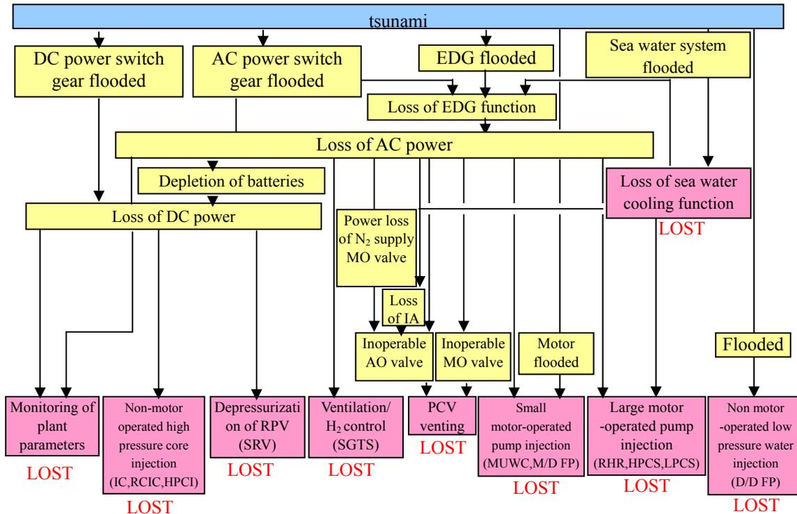
Causes leading to the loss of critical functions to prevent core damage and mitigate impacts
