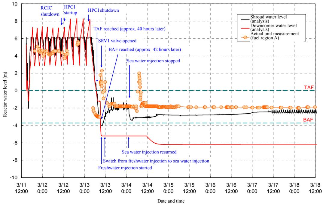
Unit 3 Changes in reactor water level [Case 1]
