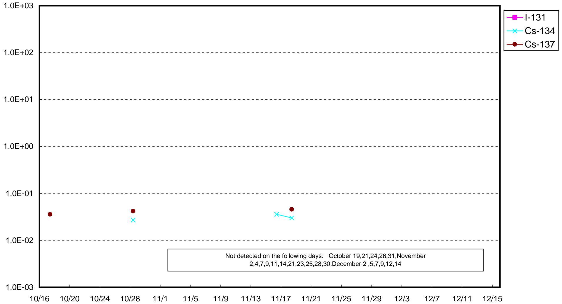
Fukushima Daiichi Nuclear Power Station : Radioactivity Density of Sub-drain at Unit 4 (Bq/cm 3 )
