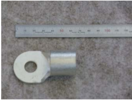
Terminals connected after treatment. Six points (3 lines × 2 (both ends)) needed connecting.
