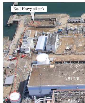
A heavy oil tank was washed away in the tsunamis up to a place near the north side of the Unit 1 turbine building.
