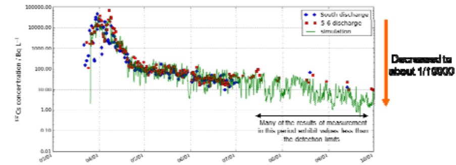
Fig.3 Concentration of radioactive materials in seawater near the water discharge canals of the Fukushima Daiichi Nuclear Power Station
