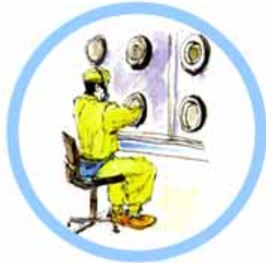
Example of a glove box Test atmosphere control, pollution dispersion prevention
