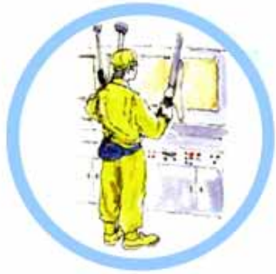
Example of a room with a high shielding function (hot cell) and remote control (manipulator)
