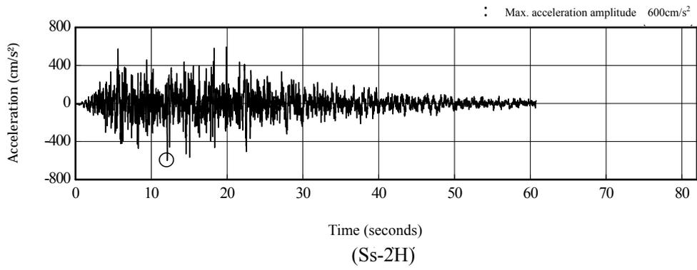
Figure-3.4.2 Time History Acceleration Wave Profile (Horizontal Direction) of Reference Seismic Motion at Location of Free Rock Surface
