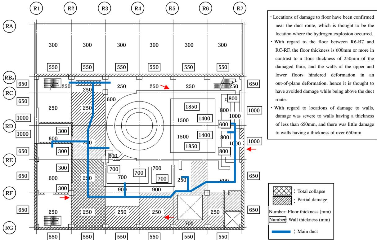
Figure-2.3.3 Damage Conditions (3<sup>rd</sup> Level)
