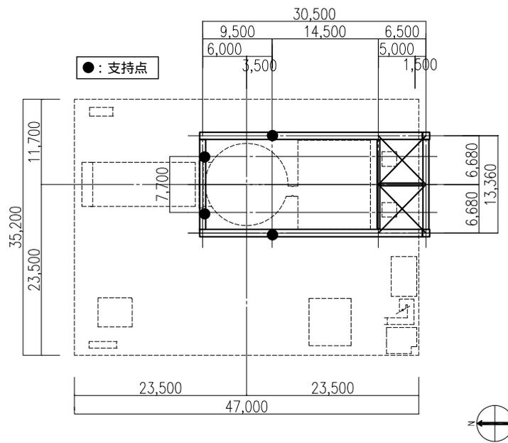
Figure-1.4.2. Beam Plan of Frame Supporting Fuel Handling Equipment (O.P.41,420)
