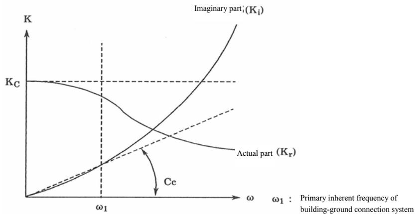
Figure-3.5.2 Approximation of Ground Spring
