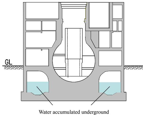
Figure-1.8.1 Illustration of Underground Accumulated Water (North-South Cross-Sectional View)
