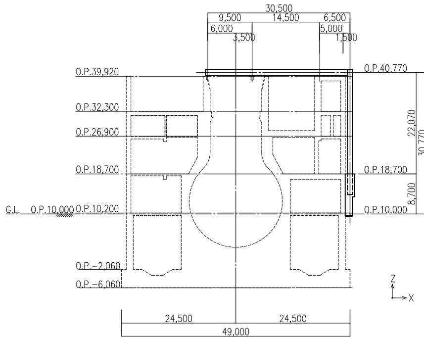
Figure-1.4.1. North-South Cross-Sectional View of Frame Supporting Fuel Handling Equipment
