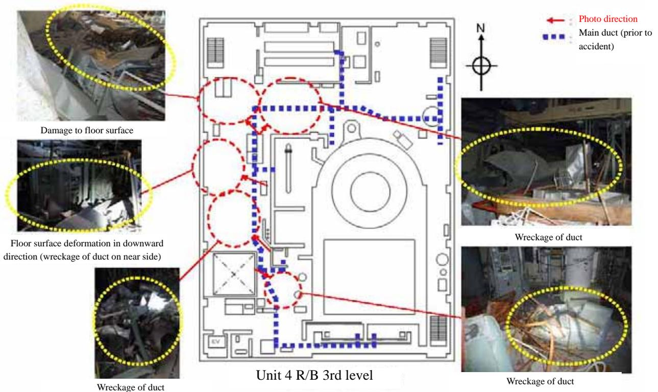
Figure-2.2.3 Investigation Results of Conditions of Damage inside Building (3<sup>rd</sup> level)
