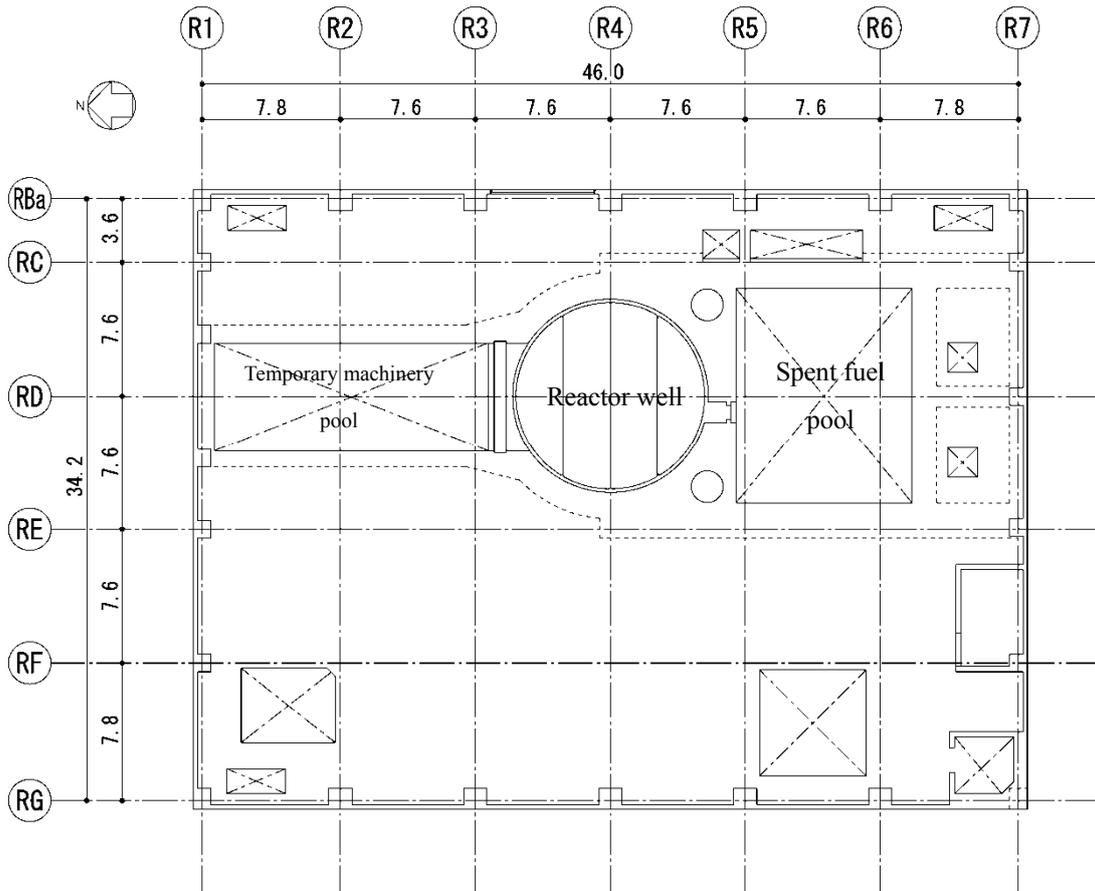
Figure-4.1.1 Plane View of 5<sup>th</sup> Level
