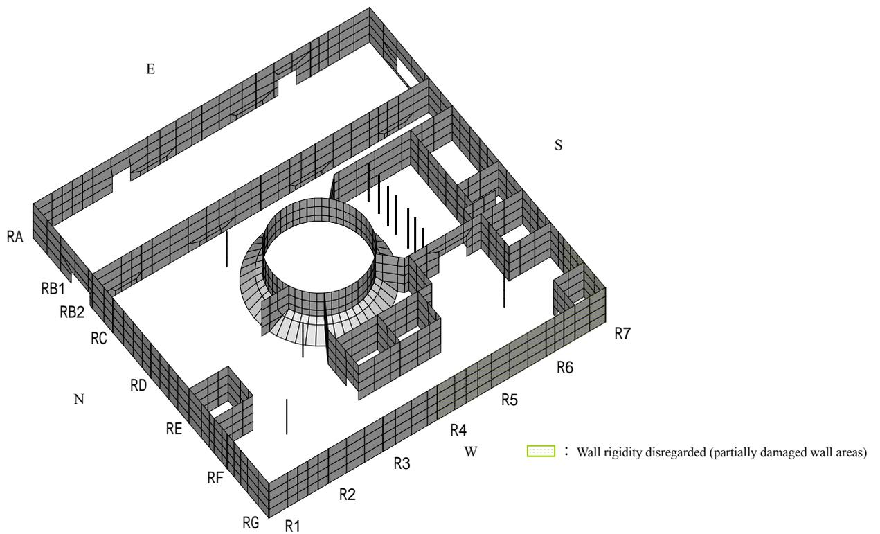
Figure 4.3.4 Damage Model: Isometric Drawing of 2<sup>nd</sup> Level (O.P. 18.7m)
