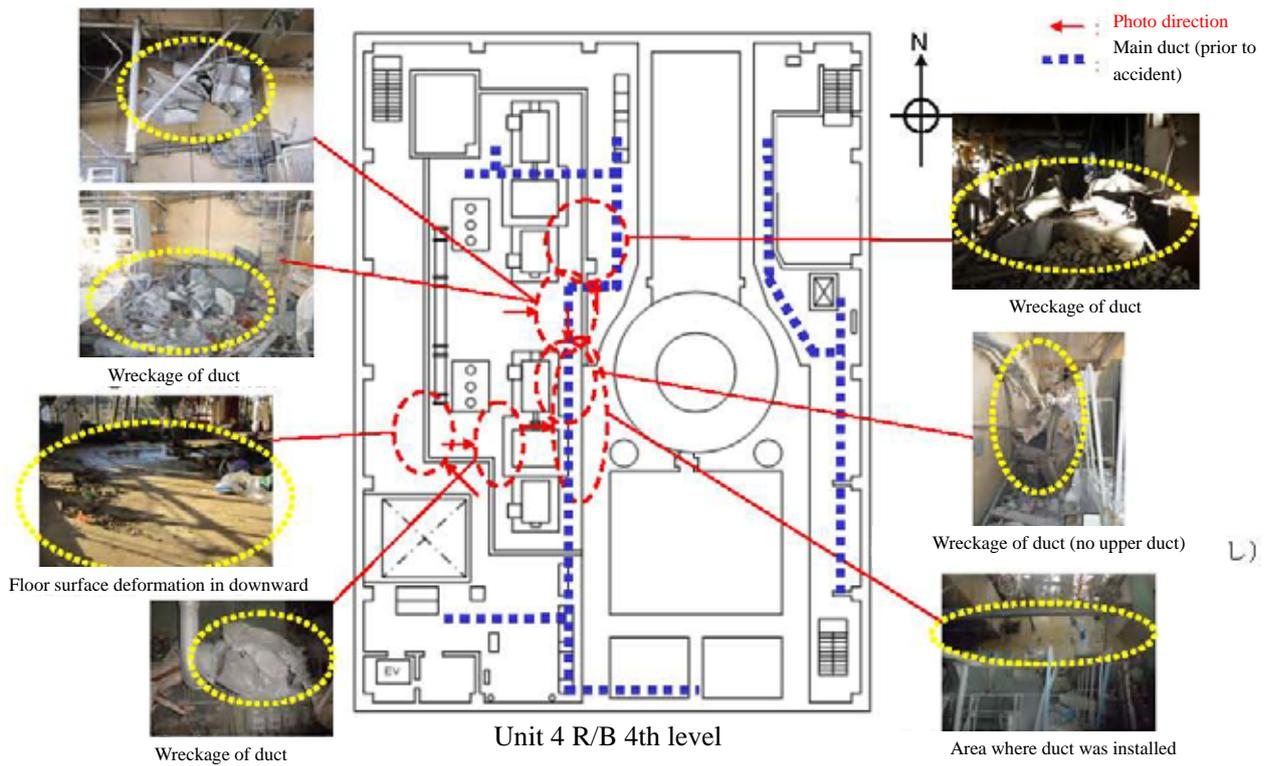
Figure-2.2.2 Investigation Results of Conditions of Damage inside Building (4<sup>th</sup> level)
