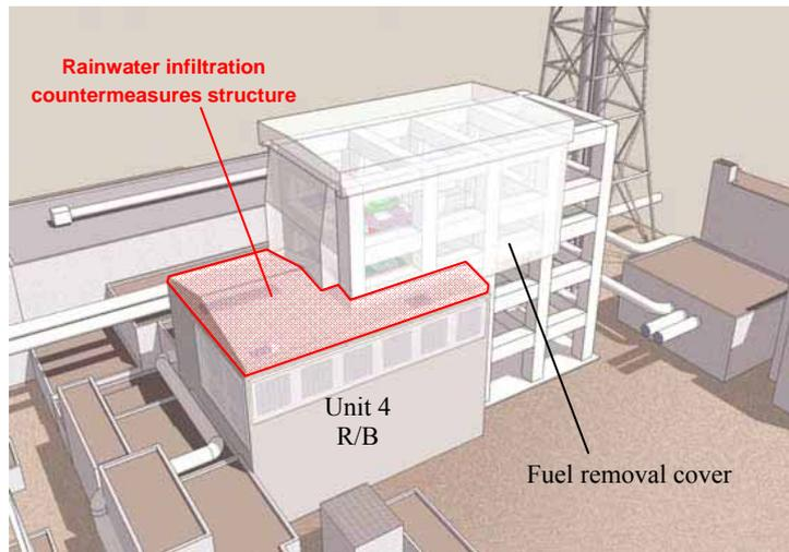
Figure-1.5.1 Illustration of Structure as Measure to Counter Infiltration of Rainwater
