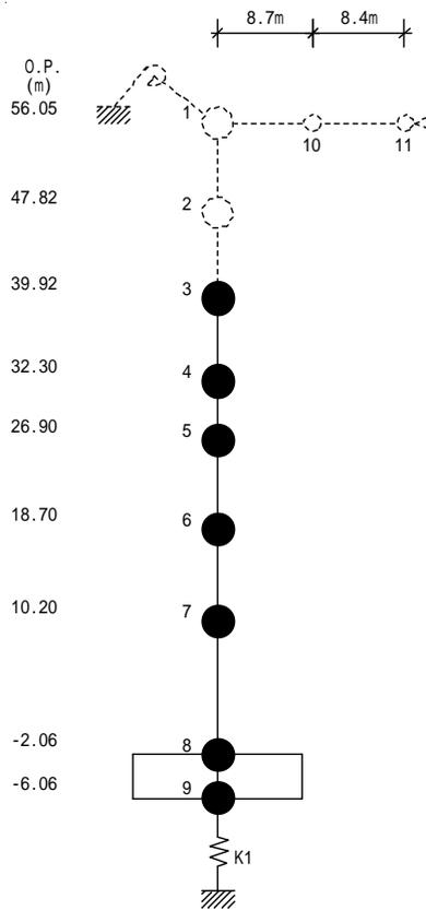
Figure-1 Building Analytical Model (Vertical Direction)
