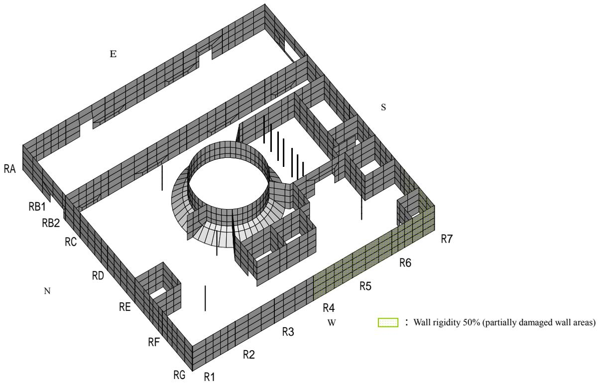
Figure-4 Damage Model: Isometric Drawing of 2<sup>nd</sup> Level (O.P. 18.7m) (Parameter Case)
