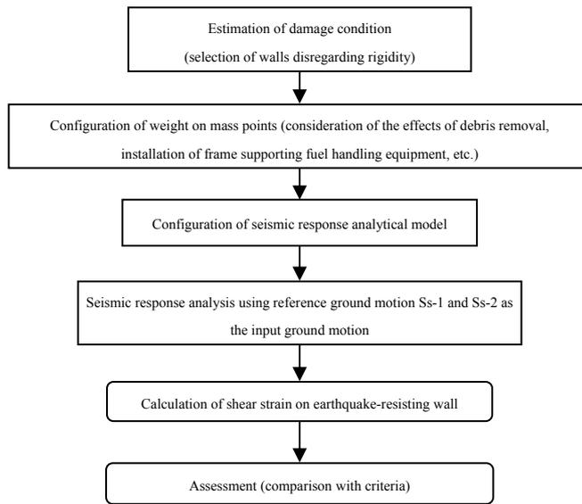
Figure-3.1.1 Flowchart of Seismic Safety Assessment of Reactor Building
