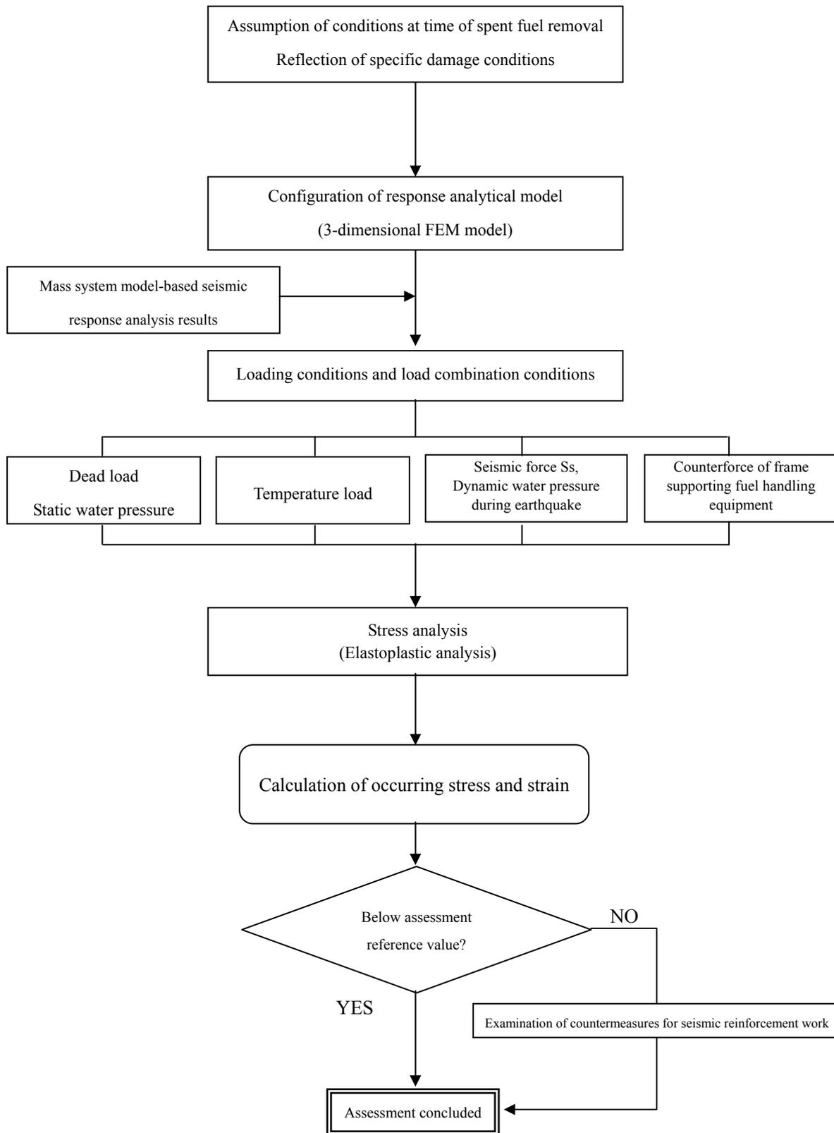
Figure-4.1.3 Flowchart of Seismic Safety Assessment of Spent Fuel Pool
