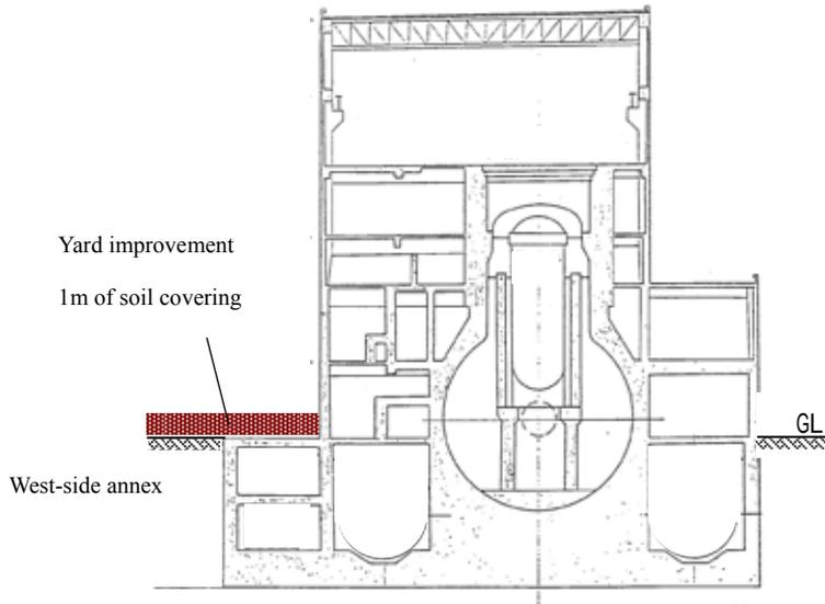
Figure-1.7.1 Illustration of Yard Improvements (East-West Cross Sectional View)
