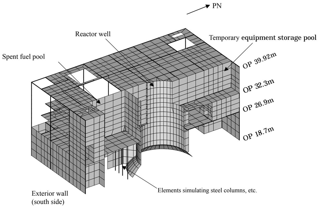
Figure-4.2.1 Schematic Diagram of Analytical Model
