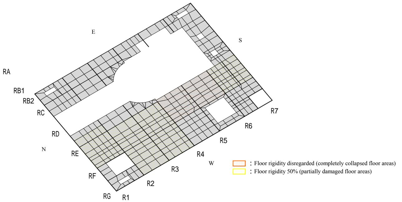
Figure-1 Damage Model: Isometric Drawing of 5<sup>th</sup> Level (O.P. 39.92m) (Parameter Case)
