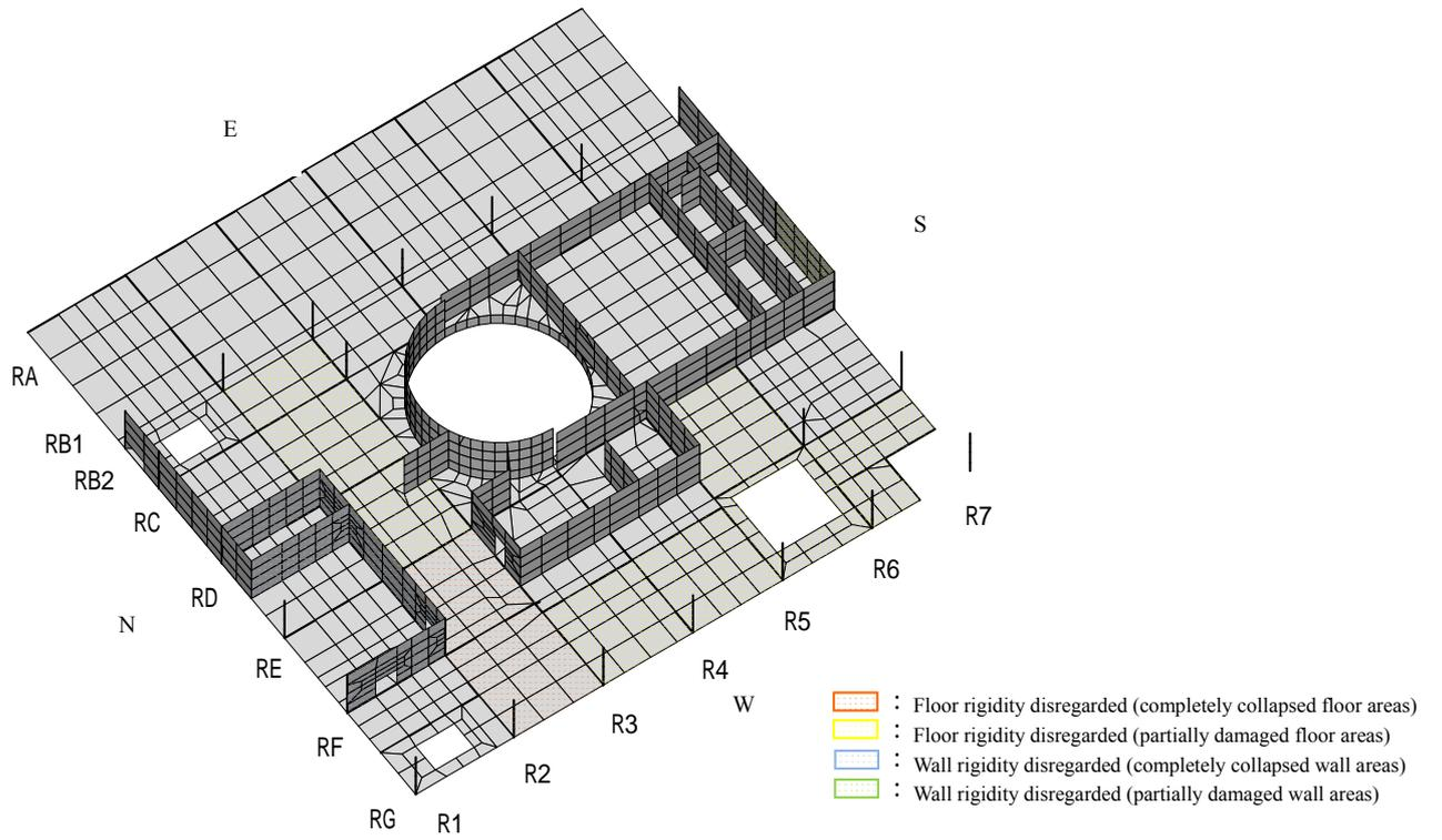
Figure 4.3.3 Damage Model: Isometric Drawing of 3<sup>rd</sup> Level (O.P. 26.9m)
