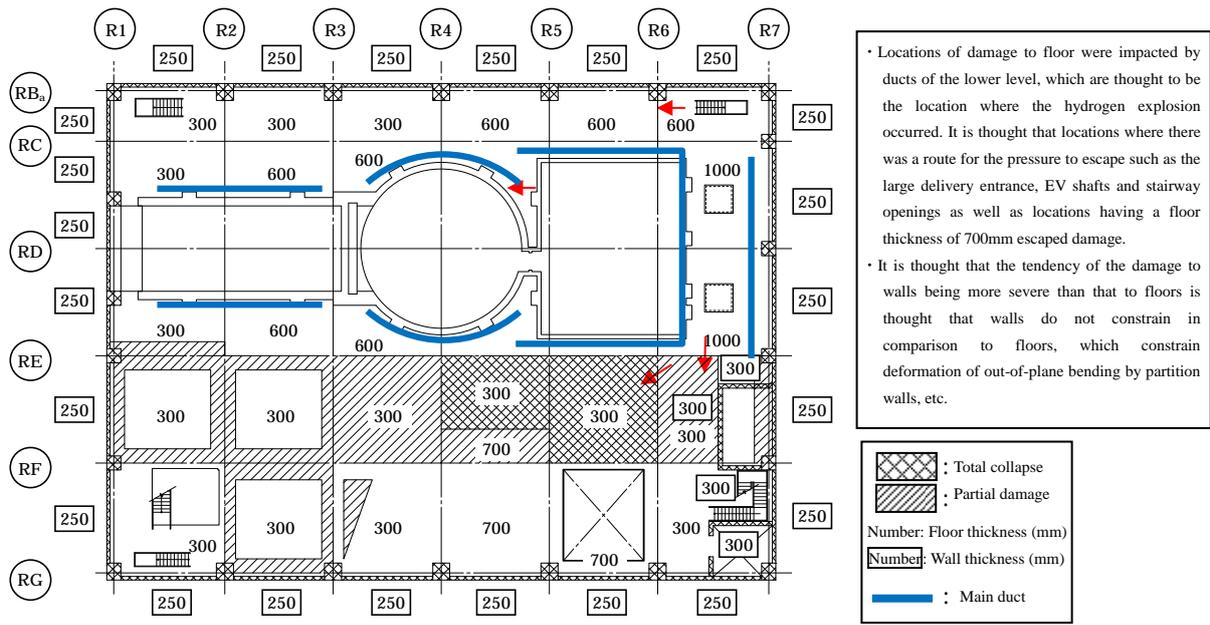
Figure-2.3.7 Damage Conditions (5<sup>th</sup> Level)
