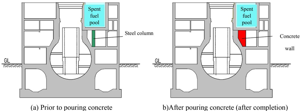
Figure-1.6.1 Illustration of Support Structure for Spent Fuel Pool Base (North-South Cross-Sectional View)
