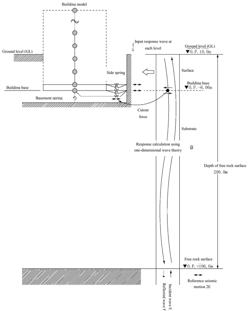
Figure-3.4.1 Conceptual Diagram of Input Seismic Motion Used in Seismic Response Analysis
