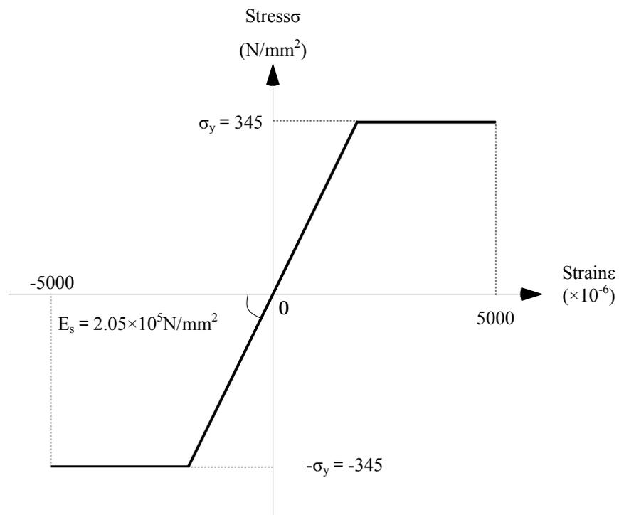
(b) Stress-Strain Relationship of Reinforcing Steel
