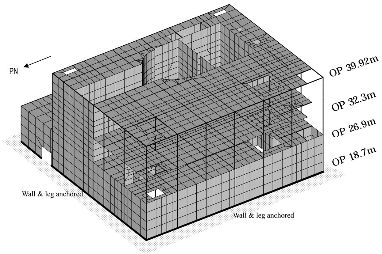
Figure-4.2.3 Boundary Conditions of Analytical Model
