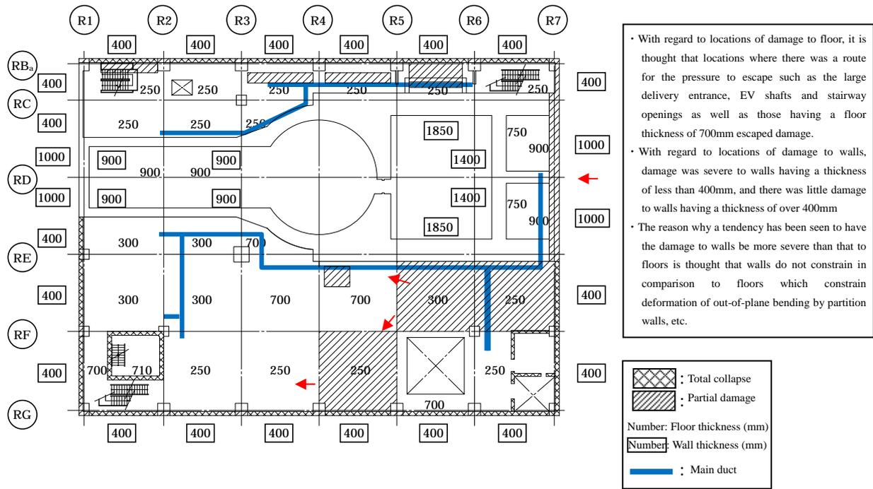
Figure-2.3.5 Damage Conditions (4<sup>th</sup> Level)
