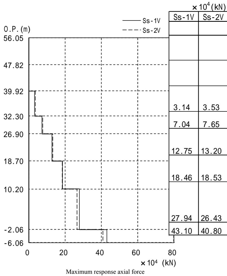
Figure-3 Maximum Response Axial Force (Vertical Direction)
