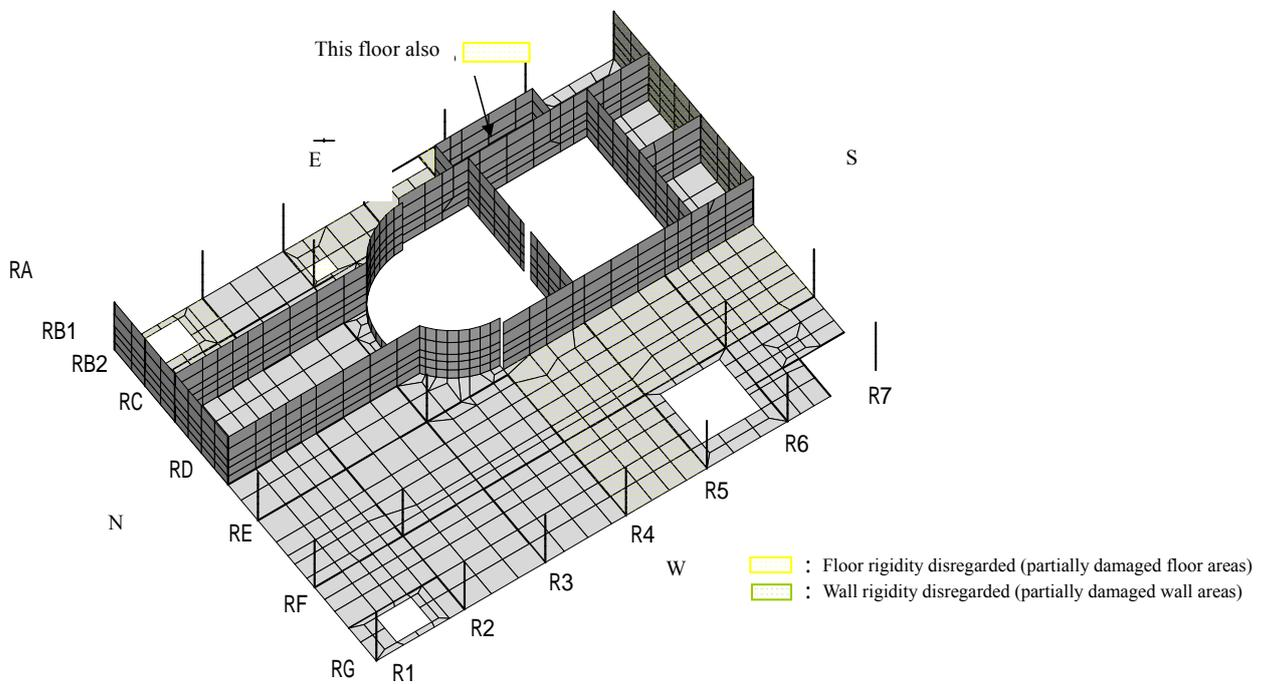
Figure 4.3.2 Damage Model: Isometric Drawing of 4<sup>th</sup> Level (O.P. 32.3m)
