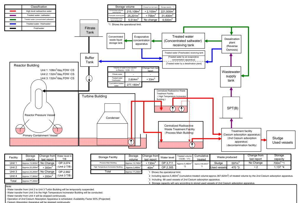
Water transfer from Unit 1 to Unit 2 Turbin Building will be conducted.
